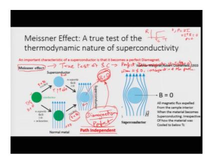
We had started taking a look at the phenomenon of super conductivity, which is the phenomenon in which if you measure résistance as a function of temperature; then below a certain temperature which is called as a super conducting critical transition temperature. The resistance goes very low, it goes below measurable values and typically it is considered it goes to the 0 resistance state.
