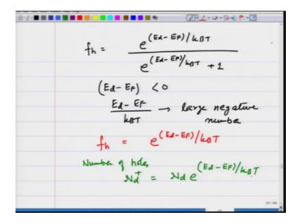
So, I get f h which is e raised to E d minus E F over k B T over e raised to E d minus E F over k B T plus 1. Now, we already said k B T is very small and E d minus E F is negative and E d minus E F over k B T is going to be large negative number. So, I can write f h is equal to E raised to E d minus E F over k B T roughly. And therefore, the number of holes at the donor level Nd plus is going to be equal to Nd times e raise to E d minus E F over k B T.
