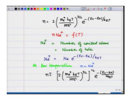
If you want to get the prefix also then I am going to have n equals 2 m e star k B T over 2 pi h cross square raise to 3 by 2 e raise to minus E c minus E F over k B T. This is the number of electrons and we are going to have n times Nd plus equals a function of
