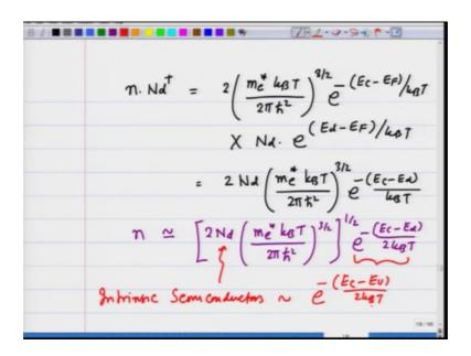
This gives me Nd plus is equal to 2 m e star k B T over 2 pi h cross square 3 by 2 times e raise to minus E c minus E F over k B T times Nd times e raise to E d minus E F over k B T which is nothing, but 2 Nd m e star k B T over 2 pi h cross square raise to 3 by 2 e raise to minus E c minus E d divided by k B T.
