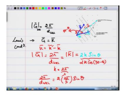
Now, with this result in mind now recall that your Laue's condition for Bragg diffraction or for diffraction of x-rays; the Laue's condition for diffraction of x-rays is G is equal to K. And here in this diagram G is equal to K; where k is the scattered wave vector minus the incident wave vector.
