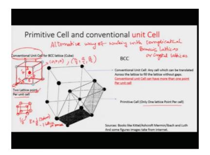
And if those are the primitive vectors, this is your primitive cell ok. If you look at your BCC lattice, you can define your primitive cell which is the smallest volume of lattice points which will have only one lattice point per cell a 1, a 2, a 3 which are the primitive lattice vectors I have already shown you. And this is the volume which is made by the primitive lattice vectors, the primitive lattice volume and it is pretty complicated. So, as
