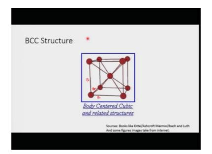
So, first we look at the body centered structure. The body centered structure as I said has atom at the corners of the cube and has a atom at the centre. And the lattice parameters are a a and a, the lattice parameters are exactly identical. So, you have atoms which are sitting on the corners of the cube, and one in the body of the cube which is in the centre of the cube and this is your body centered cubic structure.
