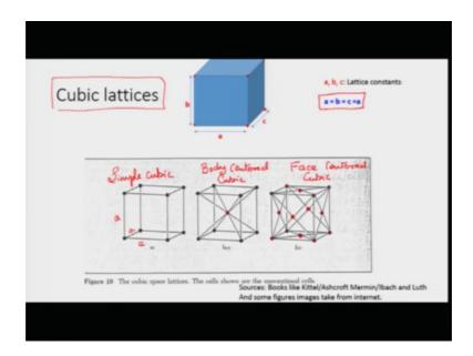
And amongst those 14 set of Bravais lattice is an important set which is falls amongst the cubic lattices. And as the name suggests the points are arranged at the corners of the cube. The spacing between consecutive lattice points is your lattice constant. And for a
