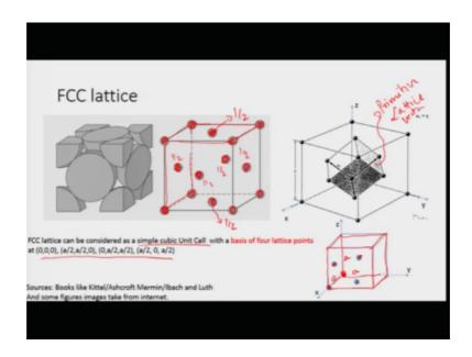
Next we go to the FCC lattice - a face centered lattice. A face centered lattice is as I had said that you have a on the faces of each cube, you have a lattice point along with points which are sitting at the corners of the cube. So, you have points which are sitting on the faces of each edge of a cube as well as on the corners of the cube. So, this is your face centered cubic structure.
