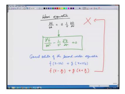
In the previous lecture, I described the wave equation starting from waves for the equation for waves travelling to the left or the right which was given by d f by d x equals plus or minus 1 over v d f by d t which was combined together to give a wave equation d to f by d x square minus over v square d to f by d t square is equal to 0 and we said the general solution is it could be the wave travelling to the right wave travelling to the left and the linear combinations.
