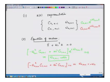
Xt representation is going to be a collection of numbers of C n, n minus 1 or C n, n plus 1 because maximum n change could be 1 and the corresponding frequency here let it be omega n, n minus 1 and omega n, n plus 1. So, that the time dependence can be written as let me write that in a different color C n, n minus 1 e raise to i omega n, n minus 1 t and the other one as C n, n plus 1 e raise to i omega n, n plus 1 t that is the time dependence.
