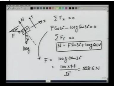
What I have is this block 100 G pulling it down, N acting this way and F in this way. Let me take this to be the x-axis and just to be the y-axis. Summation Fx is equal to 0 gives me let me make the angles, this is 30 degrees and so is this. So it gives me F cosine of 30 degrees - 100 G sine of 30 degrees is equal to 0. The balance in Y direction gives me N is equal to F sine of 30 degrees + 100 G cosine of 30 degrees.
