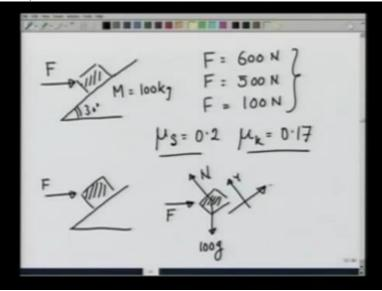
As a  $2^{nd}$  example, let us take the case where again I take a ramp at 30 degrees from the horizontal, put a block here of mass M equal to 100 kg and apply a force in this direction F. I would like to know, what happens to the block if F equals 600 newtons, if F equals 500 newtons and if F equals 100 newtons. I want to know in these 3 cases, does the block move? Does it remain stationary and so on?
