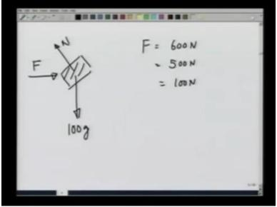
As I said earlier, there is another way of doing this problem and that would be that given this block and given this force F which could be 600 newtons or 500 newtons or 100 newtons, calculate the force required to keep the block in equilibrium and calculate the maximum possible frictional force.
