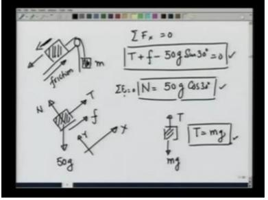
And therefore I can have a range of small mass M that would balance the bigger mass. Let us say  $1^{st}$  that I reduce this mass below 25 kg, then the bigger mass would have a tendency to move down this way. If this has a tendency to move down this way, there will be a frictional force opposing it. And this frictional force that oppose it makes it possible to have mass M much less than 25 kg and still have this block in equilibrium.
