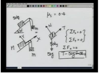
The problem I am going to solve is if I have a block of say 50 kg on a ramp with this angle being 30 degrees and let us say I tie it with a pulley and have another mass here small M, I want to know for what range of mass M would this block of 50 kg remain static on the ramp given that myu S that is the coefficient of static friction between the 2 bodies is 0.4. Why should small M have a range?
