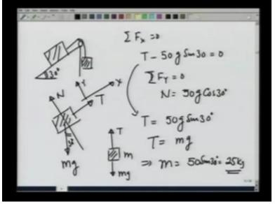
What we are doing is having a mass 50 kg on a ramp of 30 degrees, when I make the free body diagram of this big mass, it has the tension T, normal reaction N and MG pulling it down. This angle is going to be 30 degree. So summation Fx equal to 0 if I take this to be the x-axis and this to be the y-axis gives me T - 50g sine of 30 equal to 0 and summation FY equal to 0 gives me N equals 50g cosine of 30 degrees. This gives me that the tension T should be equal to 50g sine of 30 degrees.
