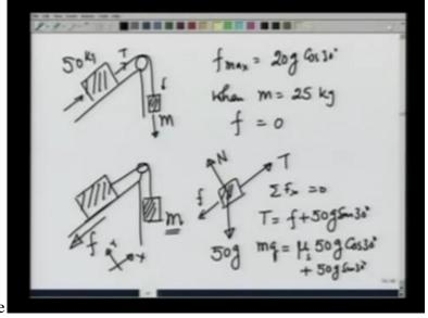
So on this ramp, this is mass M, this is 50 kg. If I have 7.68 kg, M equal to 7.68 kg, this block is in equilibrium although it has a tendency to move down. What happens when I start increasing the mass on it? So I go beyond 7.68, maybe I make it 8, 9 kgs, 10 kgs, 11 kgs and so on. When I increase the mass, I would increase the tension. If I increase the tension, I would not require that large a frictional force to keep the big block in equilibrium.
