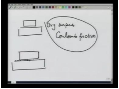
Now the frictional force could be between two dry surfaces and this is known as Coulomb friction. It could also between 2 surfaces that have a thin layer of liquid in between. There is a sort of wet friction. Friction is also present when something moves in a liquid known as the viscous force. In this lecture, we will be concerned primarily with: fiction or friction between two dry surfaces. To understand friction, let us perform a small experiment.
