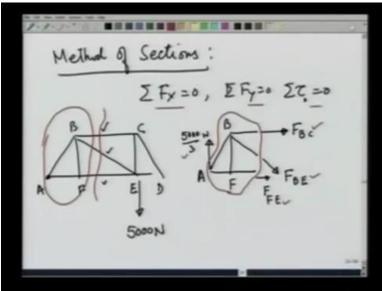
In that case, the method that is used is known as the method of sections in which case we cut a section through the truss so that maximum of 3 members are cut and then I have 3 questions to solve. Namely summation FX equal to 0, summation FY equal to 0 and summation Tao about some point equal to 0. That gives me those 3 forces. Let me illustrate this method again by the same truss that we have solved so far.
