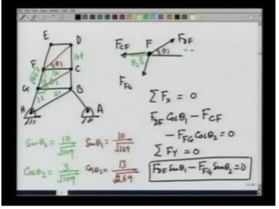
So to calculate the forces on F, let us balance the forces on F. Let me make the truss again. A, B, C, D, E, F, G, H and I have already shown you how these are the other lines. This is angle theta1. If I look at point F, it has a force EF which is 0. It has force , do I call it FD or DF? Let me see. I call it DF. FDF acting at an angle theta1 then this has a force and in anticipation I am going to make the direction down FFG and let us call this angle at which it is acting, theta2.
