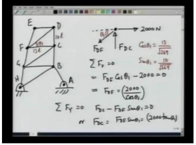
So if I go to point D, let me again make the structure. Point D, A, B, C, D, E, F, G, H. At point D, FED is 0 and there is only one load, 2000 newtons. There would be a force FDF and are vertical force. Again in anticipation, I am making it like this, FDC. There are 2 unknowns and both of these, I can determine. Let this angle be theta and that will be the same angle as this. This is 10 L, this is 13 L. Let me in fact call it theta1 because I am going to require other angles later.
