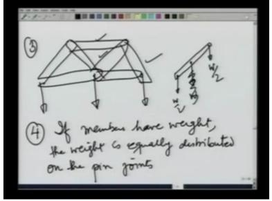
Next, we are going to assume that at any truss, all the load is going to be only on the pin joints. That is the next assumption. And finally, if members, that is these rods have weight, the weight is equally distributed on the pin joints. That is, if for example a member may have weight W, then I am going to say that this pin joint bears W by 2 and this pin joint also bears W by 2 of this weight.
