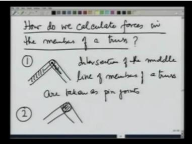
How do we calculate forces in the members of a truss. We are going to restrict ourselves to plane trusses which are the ones that I showed you and we are going to do our analysis under certain assumptions. Number 1, when these members which we take to be sort of rods but are wide enough, when the middle line wherever it cuts, we are going to to take that intersection as the pin joint.
