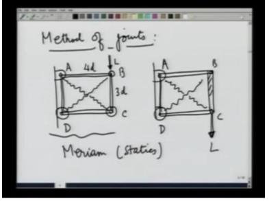
I am going to demonstrate the method of joints through several examples. As the 1<sup>st</sup> example, let me take a system, a simple system which is made of 4 rods. One fixed pin joint here. This is a rod. Another rod like this. The pin joint here. 3<sup>rd</sup> rod like this and this is on a roller, 4<sup>th</sup> rod here. And there are 2 ropes along the diagonal. Let me call this system A, B, C and D.
