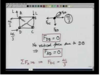
What we have is L here at point C, point A I have a force acting towards left, 4L by 3, force acting towards vertically up, L, I have a force acting on this joint in this direction, 4L by 3 and I want to calculate other forces. This is point C, this is point D. Let us take the joint D or pin at D and see what the forces on D are. Now we are really using the method of joints. Each joint we are going into bring into equilibrium by applied forces.
