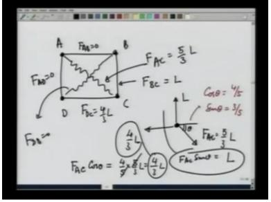
So what we have found on this frame A, B, C, D, FAB is 0, FAC is five thirds L, FDC is four thirds L, FBC is equal to L, FAD is equal to 0 and FDB is equal to 0. With these forces, let us see if point A is under equilibrium. Remember, we found that on A there is a force in this direction which is four thirds L, there is a force upwards which is L and now I know because of the tension in the rope, there is a force FAC which is five thirds L, this angle is theta.
