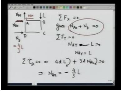
So let me make it again. There is a load L, ND, NAX, NAY. Summation Fx equal 0 gives NAX + ND equal 0 and summation FY equals 0 gives NAY equals - L. Sorry I should write NAY - L equals 0 or NAY equals L. That is it is vertically upward direction. Summation torque about D, this is point D, A, B, C is equal to 0 gives 4D times L clockwise lures 3D times NAX also clockwise, should be 0.
