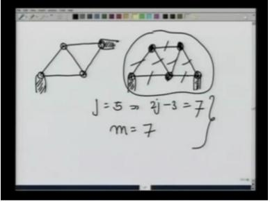
So let us see now given a basic truss like this which I just solved for, how can I make a bigger truss? Let us see, if I want to extend this further, I would apply or put a member here and give a joint here. This joint now has 3 members that can provide equilibrium. Then this point, suppose I do not want to provide a support here, I have to provide one more member and I could provide a fixed support here.
