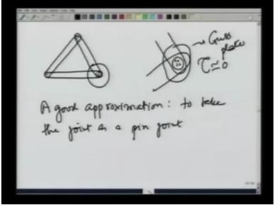
If I take these 3 rods and replace them by slightly wider members with the width of the members being much smaller than their length and instead of applying a pin joint, bolt them here, bolt them here by a plate. That is each joint here looks something like this. And I have put a plate here with bolts here. Even then, it is a good approximation to take this as a pin joint. So a good to take the joint as a pin joint.
