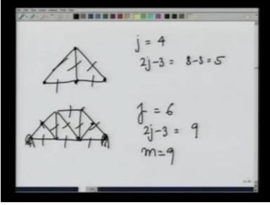
In the previous lecture, you notice that both the ants are put on a fixed point. Actually this make the system indeterminate because the number of external forces is now 4. We could make it determinate by putting the right-hand side of the system on a wheel or on roller. Let us take one example of this. And this is a very particular structure the time taking. (Refer Slide Time: 0:42)
