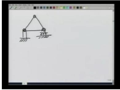
For completeness, I should point out that the triangle that we just made should actually be fixed like this on a fixed pin on the left and on a roller or a wheel on the right. This will make the system statically determinate. Through this, what I have done is, provided you an example of solving for the forces in a truss through method of joints. That is we take each joint, each pin at each joint to be in equilibrium. Now, a few subtle points about trusses. (Refer Slide Time: 11:30)
