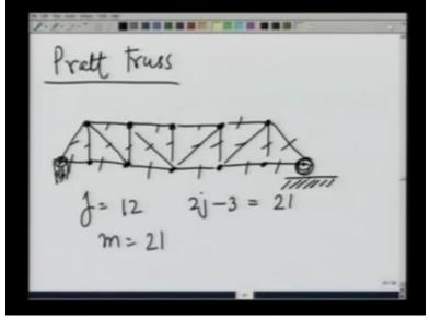
Several examples of trusses that you see in everyday life are example, Pratt truss which you see. Pratt truss which is like this. This put on the supports here and these are joints. Let us see the number of joints here are 1, 2, 3, 4, 5, 6, 7, 8, 9, 10, 11, 12. 12. So 2J - 3 is 21. Number of members is 1, 2, 3, 4, 5, 6, 7, 8, 9, 10, 11, 12, 13, 14, 15, 16, 17, 18, 19, 20, 21. So this is a statically determinate truss and capable of remaining in equilibrium.
