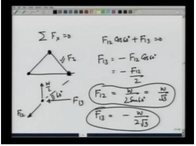
Similarly, summation Fx is equal to 0 I recall that I am talking about this pin. On this pin, there is a force this way, F 13, F 12 and W by 2. This angle is 60 degrees. I am going to have F 12 cosine of 60 degrees + F 13 is equal to 0 or F 13 is equal to - F 12 cosine of 60 degrees which is nothing but - F 12 over 2. F 12 on the other hand we found out is equal to W over 2 sine of 60 degrees which is nothing but W over root 3.
