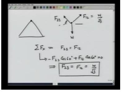
If I go to point here, then according to the way we have made forces, point 2 would be peeling a force this day which is F 23, a force this way which is F 12 which have already determined to be W over root 3 and a force this way which is W. Now summation Fx then gives you that F 23 should be equal to F 12. Of course this comes with F 23, this angle is 60. Cosine of 60 degrees with a - sign + F 12 cosine of 60 degrees is equal to 0.
