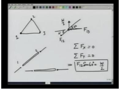
Now I know that pin1 is in equilibrium. Pin1 has a force acting on it which is W by 2. Since for the rod 12, I made forces that are pushing the rod. So the rod would be applying a force the other way on the pin. Similarly, a force on 13 that I made was also pushing the rod. That is, the force is compressive. The force that will be acting on the pin would be in opposite direction.
