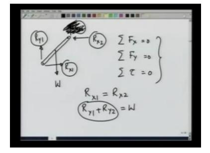
Let us look at indeterminate, corresponding indeterminate problem. If I take the same rod and put a pin joint here and also a pin joint here, in that case, this is the weight W. I will have RY1 and RX1 on the lower pin joint. RX2 and RY1 on the upper pin joint. In that case, you see that the number of unknowns are 4, RX2, RY2, RY1, and RX1. And number of equations are still 3. Summation Fx equals 0, summation FY equal to 0 and summation Tao about any point is 0.
