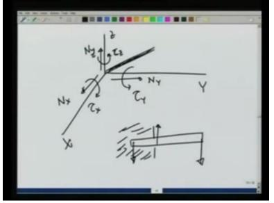
But now it can provide given X, Y and Z directions and suppose this is a fixed support, it can provide a force in X direction, it can provide a force in Y direction, and (inaudible 1:34) it can provide a force in Z direction. Since it is fixed in the wall, using arguments that we use in say 2 dimensions, it can also provide a torque about the Y direction and it can also provide a torque about the Z direction.
