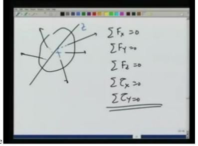
So we have a situation where all the forces are concurrent on a line. That is they all intersect one particular line which we are taking to be the Z axis. In that case, of course I have to satisfy summation FX is equal to 0, summation FY is equal to 0, summation FZ is equal to 0 and summation Tao X is equal to 0, summation Tao Y is equal to 0.
