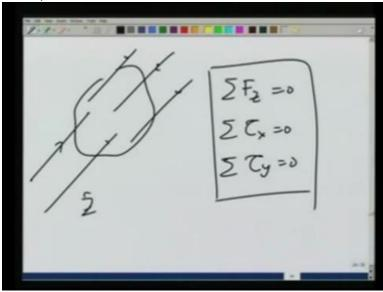
So in this case when all the forces applied are parallel and we take that parallel direction to be the Z direction. In that case, the equilibrium condition is going to be summation FZ is equal to 0, summation Tao X is equal to 0 and summation Tao Y is equal to 0. Only 3 conditions.
