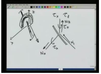
For example, suppose I were to give you a support like this with some thickness through which I put a shaft through a hole here. Now you will see, if I rotate the shaft like this, it cannot turn. If I rotate the shaft like this, it cannot turn. So if I take this to be X, this to be Y and this to be Z direction, let me be a little more careful, let me put Y perpendicular to the support like this. Then you can see that about the X axis, I cannot rotate it.
