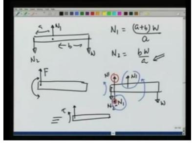
So what we find is for this built-in support, N1, N2, W. We have N1, this is B, this is A, this is equal to A + B times W over A. And N2 is equal to BW over A. I could have gotten this answer directly if I took the torque about this point. But the point I am trying to make now is going to be slightly different. I could think of this whole thing this built-in support as if it is applying a torque at this point at the end in one direction or the other and a force F.
