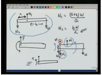
It is actually better understood if we go back to the slide and see if A is large, if A is large, I am talking about this picture, if A is large, then N1 provides a larger and larger and larger torque. And therefore, with large A I need less N1 at this point. And therefore if you want to have a very very stable support, push it really deep into the wall.
