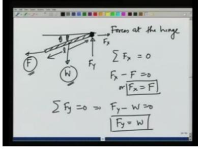
So the problem we want to solve is, suppose you pull this bus out and you are applying a constant horizontal force F like this. The weight of the bus is W and it is hinged here. I want to know the forces at the hinge. As I said just now the hinge is capable of applying a vertical force and a horizontal force. FY the vertical force and FX the horizontal force. And summation FX is equal to 0 gives me the horizontal force and that gives me FX - F is equal to 0 or Fx equals F.
