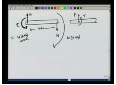
So what we say for a built-in support system is that this is capable of giving a torque and a force at this point. Of course I could have done the entire analysis about point B, this point near the wall where it enters the wall.
