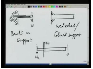
Next, we look at built in supports. That is suppose there is a support or a beam which is inserted in a wall and is like this. And I apply the load here in any direction. Or a support which is glued to a wall. Suppose I glue it here. glue or weld. So welded or glued support and this is built in support. What all are these capable of? So to understand this, let us say, I take this built in support 1<sup>st</sup> and apply a load here.
