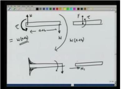
Let us see now a similar support which is not into the wall, which is not built in but is welded at the corners and I apply a load here. Let us see what will happen. As this load is applied, you will see that this has a tendency to turn like this and therefore there will be a force generated in this direction, let us call this N1. And there will be a force generated in this direction, let us call it N2.
