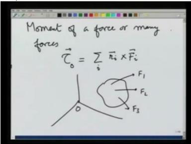
We have been learning about the moment of a force or many forces. What we have learnt so far is that the torque about origin O so that I will indicate by this is RI cross FI where we are applying these different forces F1, F2, F3 and so on about point O. We have also learnt that the torque is origin dependent.
