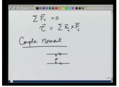
There is a very special case when the total force on the body is 0, then torque is independent of the origin. No matter about which point it is taken, it comes out to be independent. Then as a very special case of this, we define a couple moment which is nothing but two equal and opposite forces separate by a distance D. In this lecture, we study moment a little more. We will define the moment of a force or a torque about an axis.
