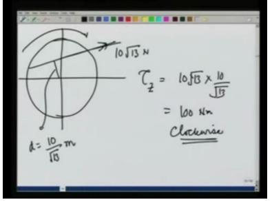
So we have F, we have D and therefore, the moment can be found out. The force is like this whose magnitude is 10 square root of 13 newtons. We have found this distance which is D is equal to 10 over 13 m. And therefore the torque about axis Z is going to be 10 root 13 times 10 over root 13 which is 100 Newton metres.
