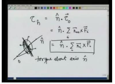
And define the torque about an axis in a slightly different manner which I will show through an example is equivalent to what you have been learning. So let us say that is a disc which is rotating about a fixed axis which is in the direction of a unit vector N and there are various forces working on it. Then the torque about the axis N is going to be equal to the dot product of N with respect to the total torque about said the origin O.
