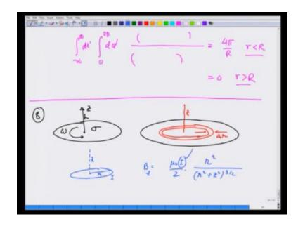
And therefore, the answer I have is therefore, that integral minus infinity to infinity d z prime integral d phi prime 0 to 2 pi. All that, that I have written is going to be 4 pi over R for r less than R and 0 for r greater than R and that is the answer. Next question number 8, a disc with it is center at the origin. Therefore, this is the z axis carries the uniform surface charge density sigma and is rotating with angular speed omega.
