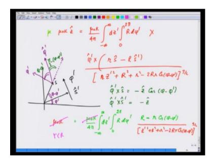
So, I am left with B which is mu 0. Let me write mu 0 k in the z direction is equal to mu 0 k over 4 pi integral d z prime from minus infinity to infinity, integral R d phi prime from 0 to 2 pi times phi prime cross r s minus R s prime divided by z prime square plus R square plus r square minus 2 R r cosine of phi minus phi prime raise to 3 by 2. Let us see what phi prime cross s is. So, let us just look on this x y plane, let us say this is s prime, this is phi prime and this is s.
