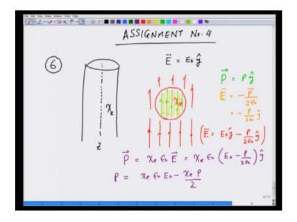
We have been solving assignment number 4, and we have solved problems 1 to 5, so we now solve problem number 6, which says consider a long cylinder with it is axis on the z axis. So, we have a long cylinder, so that fringe effects are gone with it is axis on the z axis. It is made of a dielectric material of electric susceptibility chi e, if it is put in a uniform electric field E equals E 0 y, find the electric field polarization and displacement in the cylinder.
