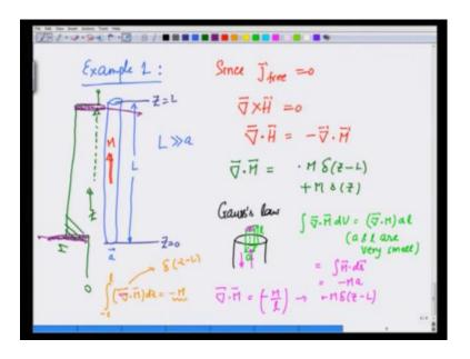
Let us take a few examples. Example one: suppose I have a long bar magnet, its length is L and radius a, such that L, or let me make L properly. The total length is L. L is much, much greater than a. So, I can ignore the fringe effects. And this carries a magnetization M along its length. Since j free is 0, I have curl of H is equal to 0 and divergence of H is equal to minus divergence of M. Let us see what divergence of M in this case is going to be.
