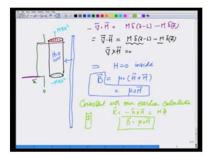
I have this long; and I am making a slightly different picture, so that you can see it clearly. A long bar magnet on which the magnetization goes down is M throughout the magnet and goes down again; 0, M. And its divergence has this delta function here and delta function here.
