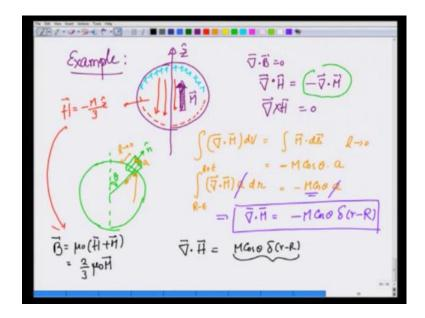
Let me do another example. A well-known example that we have been treating. And I said that this becomes nice example for magnetic field. In this example, I will take this magnetized sphere, which has magnetization; these are directions, this is magnetization M.
