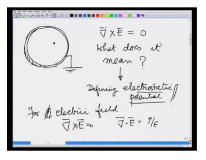
This need not be the case; for example if I take a charge say inside a grounded sphere. Then, this charge, since this is shielded by a metallic grounded sphere. It need not give a field which is given by the previous formula. And therefore, what one needs to do is solve those differential equations with the boundary condition, appropriate boundary condition, we will talk about it a little more little later.
