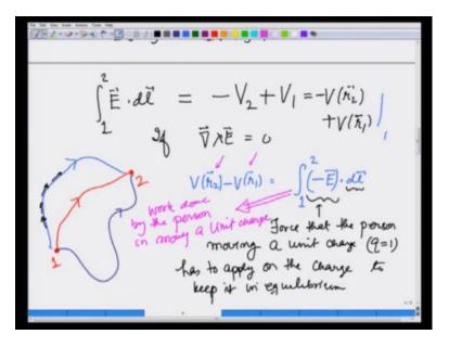
So, curl of 0, we have seen tells me that, if I travels between two points 1 and 2, the integral is independent of the path. And therefore, I can write E dot d l between two points 1 and 2 is independent of path and I am going to write this in a particular way, I will write it as minus v 2 plus v 1, if curl of E is 0. Let us understand, what these v's stand for and also write this in a better way, v at r 2 plus v at r 1.
