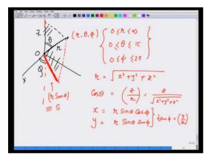
In a spherical coordinate system, a point is specified by it is distance from the origin, which I will call r and if I make the plane containing this point and the z axis. So, this is r, the distance from the origin to the point. In this plane, if I measure the angle from the z axis to this line joining origin and the point, this angle is given as theta and the angle in this plane, this entire plane, this entire plane makes from the x axis is known as phi.
