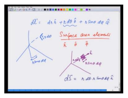
So, what is the line element that I get? I get the line element d l is equal to d r in r direction plus d theta times r in theta direction plus r sine theta d phi in phi direction. That makes perfect sense, because if I look at the coordinate system, if I move in r direction, this distance is d r, if I change theta, this distance becomes r d theta. So, that is this line element and if I change phi, the distance I cover in phi is going to be r sine theta d phi. So, this is a line element.
