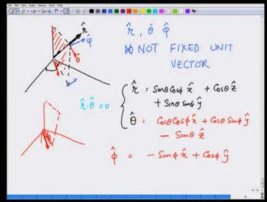
How about the unit vectors? So, I am going to have unit vectors in direction r like this. In direction theta, which is going to be in this plane containing the point on the z axis, it is going to be perpendicular to the r and like this. If I transport it parallel to itself, it is going to be pointing down like this and phi vector is going to be like the cylindrical coordinate phi vector like this, which is perpendicular to r theta and phi.
