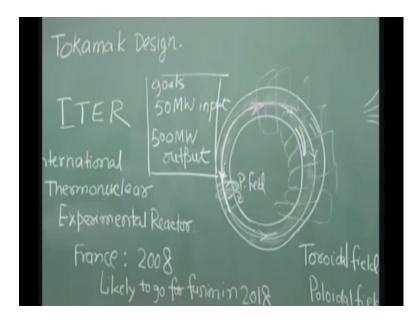
So, this I T E R the goals is that 50 Megawatt input and then 500 Megawatt output so, 10 times. So that is the kind of design have been created to all simulation on all calculation, on the all equations and this and that, it is still experimental reactor International Thermonuclear Experimental Reactor is still not a commercial units to produce electricity.
