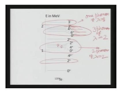
This will be true for all the nuclei, which follow vibrations, this is 2 plus and then this is 0 plus, 4 plus and 2 plus. So, this energy, these energies are roughly the same, these three and double of the first 2 plus.
