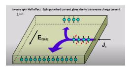
And you also see that this is called the I shear the inverse spin Hall effect this is a sample and then there is a spin polarized current if you send a spin polarized current which is shown by Js that gives rise to the transverse charge current flowing into the sample okay. So that's called I shear or inverse spin Hall effect all right. So these are very short introduction of the Hall effect let us do some calculations in order to understand things better and in a more detailed manner.
