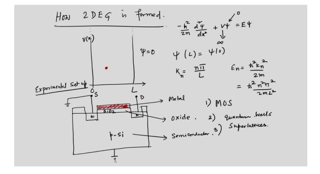
So there is a metal oxide so there is metal here so this red is metal this is an insulator called as an oxide and this is a semiconductor and that's why it's called as a MOS device metal oxide semiconductor device you know the so these MOS structures and there are quantum wells where you confine it again in the Z direction and make the electron or the
