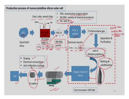
So, let us now learn how this PV cells are manufactured, which is very, very important. Because see what we know, this silicon is the second most available element in the earth, after oxygen. So, the kind of form we will get is a silicon dioxide  $SiO_2$ . So, once we have  $SiO_2$  then, what we need to do for production of these cells, first this has to be melted in a furnace, normally this arc furnace is used and at a temperature of 1900 °C.
