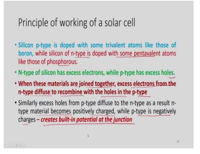
So, what we can say this silicon p-type is doped with some trivalent atom like boron, and while n-type is doped with some pentavalent atoms like phosphorous. So, this n-type silicon has excess electrons and p-type has excess holes. So, when these materials are joined together, excess electrons from the n-type diffuse to recombine with the holes in the p-type.
