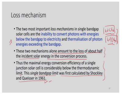
So, let us now discuss something on loss mechanism. So, as far as last mechanisms are concerned, we will have two most important loss mechanisms in single band-gap solar cells. Number one, is inability to convert photons with energies below the band-gap of electricity. And the second one is thermalization of photon energies exceeding the band-gap.
