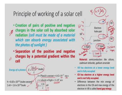
So, now let us now learn the principle of working of a solar cell. How does a solar cell works? So far, we know the construction and then know how the solar cells are manufactured. Now, we would like to know how the solar cell works. What is the working principle?
