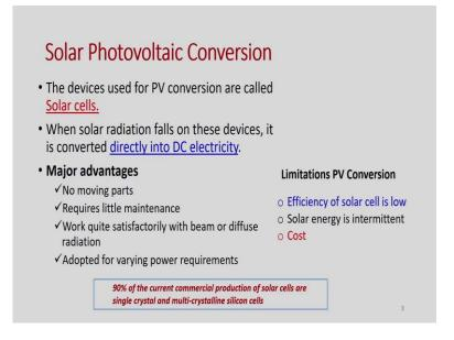
So, let us learn about solar photovoltaic conversion. So, most of the time, we heard the word solar cells. So, what is solar cells? The devices used for PV conversion are called solar cells. When solar radiation falls on these devices, it is converted directly to DC current, DC current means direct current.
