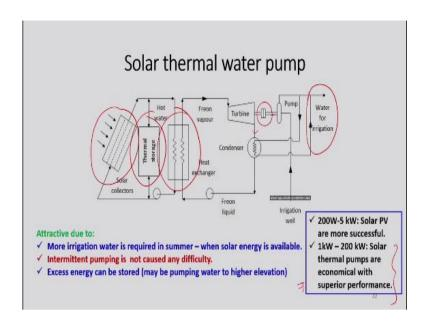
Also, we can use solar thermal energy for water pumping. So here, similar configurations we have. So, we have flat plate collector, we have storage tank and of course, we need to have a heat exchanger to exchange the heat from the water to the working fluid used in the organic rankine cycle and we can generate electricity. So, once we have generated electricity, that can be used to pump water and part of the water can also be used to condense the fluid coming out from the turbine.
