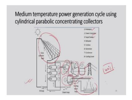
So, as far as medium temperature power generation cycle is concerned, we can go for cylindrical parabolic concentrating collectors. Or we can say, this is solar collector field and here, we will have this 1 is for preheater, 2 is for steam generator, 3 is for super heater and then we will have regenerator, then it will go to the turbine and then we will have generator and then we can distribute the energy in the grid line and we must have a condenser here.
