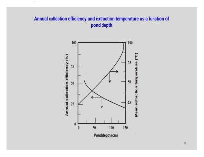
And also, we can develop the annual collection efficiency and extraction temperature, which is function of pond depth. So, this figure shows about the variation of annual collection efficiency with pond depth. So, this is something like this. So, as pond depth increases, annual collection efficiency actually increases and this mean extraction temperature is decreases with increase in pond depth.
