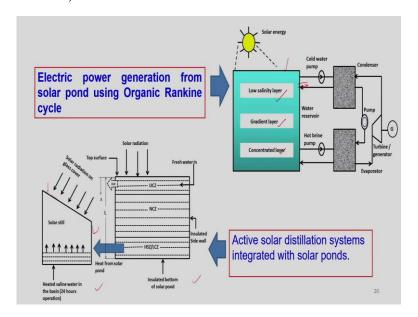
And here, what we can see is the electric power generation from solar pond using Organic Rankine Cycle. So, here is the low salinity layer, then gradient layer, then concentrated layer. What happens here, so sometimes, we have to apply freshwater and then when we have to take this saline water out and it contains saline or, say, salt and that has to be separated and
