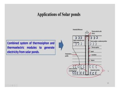
So, there are applications of solar ponds, like we can have combine system of thermosiphon and thermoelectric modules to generate electricity from solar ponds. So here, what happens, this is the thermoelectric part. This temperature difference is utilized to generate electricity and this is the collection and storage part, from useful heat gain can be extracted and applied as per the application.
