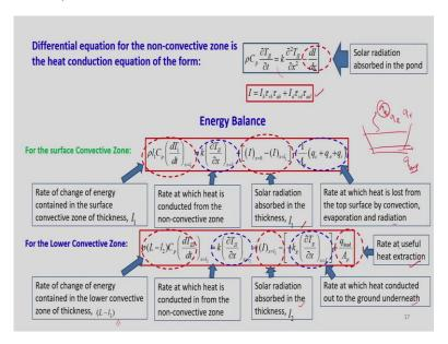
So, if we develop the differential equation for non-convective zone, it is represented something like this. So, this dI/dt is the solar radiation, which is absorbed in the pond. And this is the amount of energy which is stored, and this is the conductive heat transfer in the non-convective zone. And this I can be represented by using this expression, already this is done in the problem, what we have discussed.
