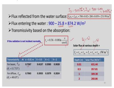
So, this is flux reflected from the water surface. So, how we can calculate? We know this  $\rho_b$  know and  $\rho_d$ , and  $I_b$  is known because  $I_g$  is given.  $I_g$  is given as 900 W/m², so what will be  $I_b$ ? So,  $I_b = (900 - 200)$  because  $I_d$  is given as 200 W/m². So, it will be 700 W/m². So that way, we can get what is  $I_b$ .  $I_b\rho_b + I_d\rho_d = 700 \times 0.2 + 200 \times 0.059 = 25.8W/m²$ .
