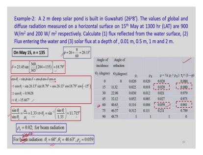
Now, let us take an example, it goes something like; a 2 m deep solar pond is built in Guwahati. Its latitude is given 26° 8′. The values of global and diffuse radiation measured on a horizontal surface on 15<sup>th</sup> May at 13:00 local apparent time or solar time are 900 W/m² and 200 W/m² respectively. Calculate number 1, flux reflected from the water surface; number 2, flux entering the water, and number 3, solar flux at a depth of 0.01, 0.5, 1, and 2 m.
