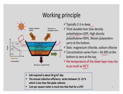
So, this is the pond. So, this the upper temperature and concentration. And what happens here, sometimes we need to provide fresh water here to maintain the salinity gradient. So, when we provide fresh water, along with this salt is also moves. Salt is also moves, and then in order to use this salt again, then we need to have a separate plant to evaporate the water present, and then we can separate salt and water, and then that salt can be used here again to maintain the salinity gradient.
