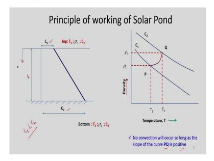
Now, let us learn the working principle of solar pond. How does a solar pond works? So here, what is shown, let us consider a pond of depth L, so it is going towards x direction and this the depth of the pond L. And let us consider, the concentration of the top layer is  $C_1$  and concentration on the bottom layer is  $C_2$ . So, there is a concentration gradient. So,  $C_1 < C_2$ , concentration of brine.
