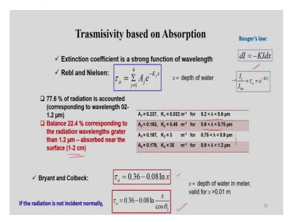
Now, let us analyze on transmissivity based on absorption. As we know, this expression Bouger's law,  $dI \propto I dx$ , and this K is the constant. This is known as extinction coefficient and we can have a solution of something like this. So, we can get the value of transmissivity based on the absorption by using this expression. But this cannot be used directly here because this K, extinction coefficient is a strong function of wavelength.
