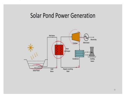
And this arrangement, what is shown here is use of solar pond for power generation. So, here what happens, collection and storage will be there and then we can circulate cold brine and then hot brine will move out and there will be heat exchanger. Heat will exchange from this hot brine to the organic fluid used in the secondary cycle. So, this may be ammonia.
