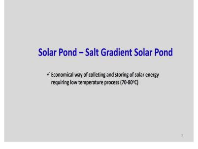
This Salt Gradient solar pond is an economical way of collecting and storing of solar energy requiring low-temperature process, and it can provide process heat at a temperature of 70 to 80 °C in an average. So, first let us learn what is solar pond?
