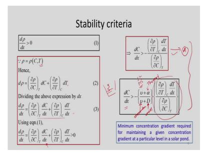
Now, mathematically, we can represent this  $\frac{d\rho}{dx} > 0$ ; that means what, density at the bottom layer is always more than the just above layer. So, this  $\rho$ , density of the brine solution is a function of concentration and temperature. So, we can apply the total differentiation  $d\rho = \left(\frac{\partial \rho}{\partial C}\right)_T dC + \left(\frac{\partial \rho}{\partial T}\right)_C dT$ . Then if we divide the above expression by dx, so it will be something like this.
