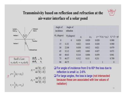
Now, let us analyze the performance of a salt gradient solar pond. So for that, we need to understand the transmissivity based on reflection and refraction at the air-water interface. Because we have air and water, this is the pond and we have air here and we have water here. So, this is the air-water interface. So, we need to know the transmissivity based on the reflect on reflection, and also transmissivity based on refraction.
