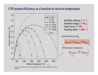
And this slide shows the efficiency vs receiver temperature. So, this is the system efficiency and this is the receiver temperature at different concentration ratios. So, these are different concentration ratios. So, it goes maximum and then it come back to 0. So, it shows the variation of efficiency with respect to receiver temperature at different concentration ratios.
