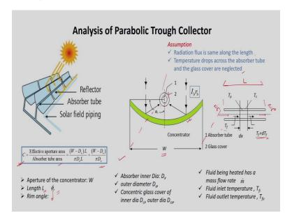
So, now let us pay attention about the analysis of parabolic trough collector. So, let us consider this configuration. So, we will have solar field, then you have absorber tube and then reflector. So, if we take a section, so it appears like this, so this is concentrator and this is the receiver system. So, when we call receiver system, it includes absorber tube plus this glass cover, which is placed concentrically and vacuum is maintained in between this.
