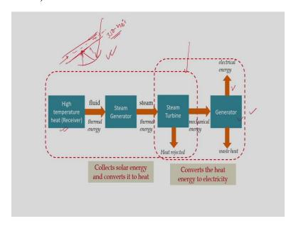
Now, let us see this picture how this high temperature heat which is generated in the receiver system. So, as we can see thermic fluids are used in the tube through which heat exchange takes place. Solar radiation, so may be this is the collector, so radiation falls here, beam radiation falls here and strikes in the receiver system; so heat transfer fluid flows.
