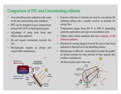
So, this slide shows about the comparison of flat plate collector and concentrating collector. As already we are aware that, this flat plate collectors are normally used for low temperature applications. So, maximum may be 100, 110 °C. For this kind of configurations, for concentrator, it may go up to 3500 °C, starting from 260 °C.
