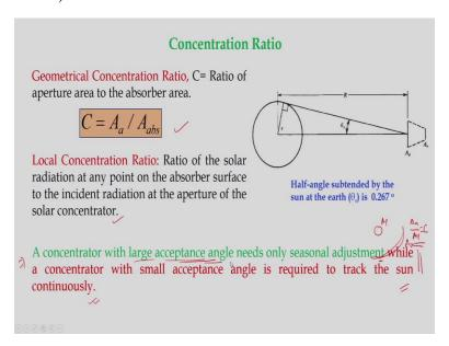
So, let us define concentration ratio. So, how we can define concentration ratio? Concentration ratio is the ratio of aperture area to the absorber area. So, as I am writing this again and again, so this is an aperture area, so maybe  $A_a$  I can write and this is the absorber area, so this  $\frac{A_a}{A_p} = C$ , which is concentration ratio. The local concentration ratio can also be defined which is the ratio
