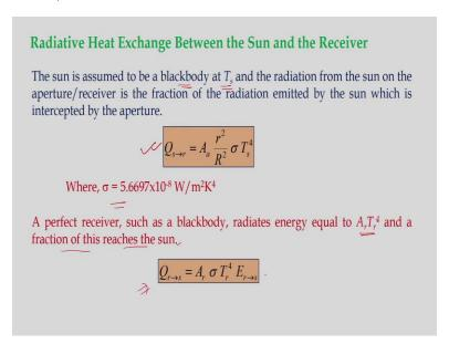
Now, let us see the radiative exchange between the sun and the receiver. So, if we consider a black body, sun is always considered as a black body having temperature  $T_s$  and the radiation from the sun on the aperture or receiver is the fraction of the radiation emitted by the sun which is intercepted by the aperture, which can be represented by this expression,  $Q_{s\rightarrow r} = A_a \frac{r^2}{R^2} \sigma T_s^4$ .
