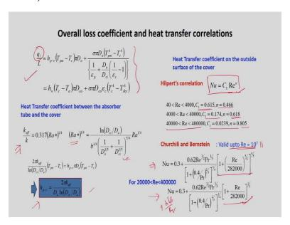
So, now next phase is how to calculate the heat transfer coefficient. So, once we know those values, instantaneous efficiency value,  $F_r$  value, F' values and then useful heat gain, then we need to know the heat transfer coefficient. How this heat actions is taking place from the collector to the absorber, then absorber tube to the glass tubes and then fluid? So, all the things we need to calculate.
