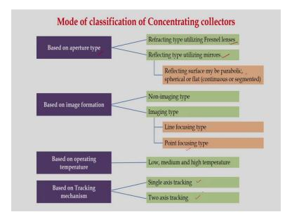
So, let us classify the concentrating collectors, there are different modes of classification. So, based on the aperture type, it's a reflecting type utilizing Fresnel lens or refracting type utilizing mirrors. So, if we have to use mirrors, then refracting surface may be parabolic, spherical or flat; that may be continuous or segmented.
