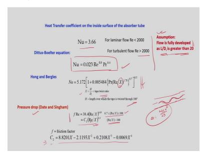
So, this heat transfer coefficient on the inside surface of the absorber tube if I am interested to know, then we need to go for this kind of correlation. Nu = 3.66, for the flow having Re < 2000. So, if the flow is turbulent having Re > 2000, then we need to use the correlations developed by Dittus-Boelter, which is something like this,  $Nu = 0.023 \,\mathrm{Re}^{0.8} \,\mathrm{Pr}^{0.4}$ .
