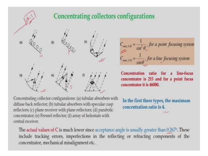
Now, let us pay attention about the different configurations of concentrating collectors. As you can see, these are tubes and one reflector is placed at the bottom of the tubes. And this is one more configurations, which is nothing but tubular absorber with specular cups reflectors. So, this kind of configurations are there to increase the concentration ratio.
