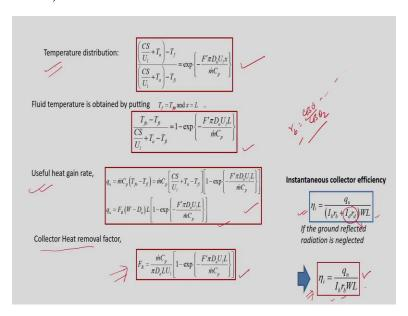
So, once you do it then we will get temperature distribution of something like this. So, fluid temperature is obtained by putting  $T_f = T_{fi}$  and  $x = x_o$ , so this should be  $T_{fo}$ . So, if x = L, the  $T_f = T_{fo}$ . So, if we substitute this, then we can have this kind of configuration.
