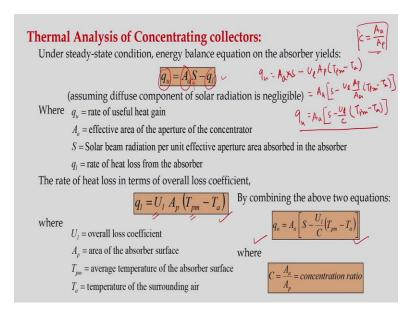
Now, let us pay attention about thermal analysis of concentrating collectors. So, under steady state condition, the energy balance on the absorber plate can be written as something like this. So, this  $q_u$  is the useful heat gain and  $A_a$  is the effective area of the aperture of the concentrator and S is the solar beam radiation per unit effective aperture area absorbed in the absorber and  $q_1$  is the rate of heat loss from the absorber.
