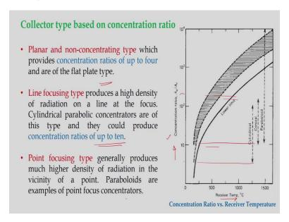
And this slide shows the collector type based on concentration ratio. So, as we can see this planar and non-concentrating type, which provides concentration ratios of upto 4 and are of flat plate type. So, if you see this figure, this vertical axis shows concentration ratio and horizontal axis shows receiver temperature. So, these are the lower limits and this is the band. Normally, this is the band at which the concentration ratio falls, when temperature increases.
