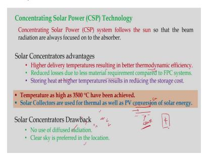
So, there are some advantages of this kind of technologies. So, first is, it is a better thermodynamic efficiency; because its operating temperature is higher or range of temperature is higher. And less material requirement compared to flat plate collector and reduced storage cost. So, these are the primary advantages of these solar concentrating collectors.
