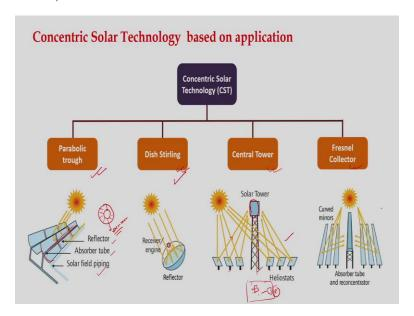
Now, let us see different CSP technologies what is available. So, first technology is parabolic trough, then dish stirling, central power receiver system, then Fresnel collector. So, what we can see here, so this is a concentrator, this part is concentrator and this is receiver system. So, solar radiations falls here and is reflected to this focal axis. So, reflector, then absorber tube, then this is solar field piping.
