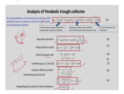
So, this energy balance on an elementary slice of the absorber tube at the distance x from the inlet. So, this gives a relationship of something like this. So,  $q_u$  is the useful heat gain which is equal to  $I_b \times r_b(W-D_o) \times \rho \gamma \times (\tau \alpha)_b$ , because beam radiation is only employed.
