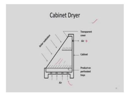
So, this is a cabinet dryer. So, solar radiation is falling, through this glass cover, and materials to be dried, we will keep here in these trays. So, these are trays, so long trays, so different stages are there for keeping the products, and air is supplied from the bottom. So, finally air has to be take out, so it will carry the moisture. And this can be taken out with time if we know the drying time for a particular material.
