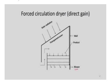
So, Forced Circulation Dryers are something like this, they have glass cover, solar radiation is falling through this glass cover, and materials to be dried, we will keep in these trays, and blower is employed here to suck the air, because it is a active device, so external unit has to be employed to suck the air. So, drying is performed by using this sucking effect of this air.
