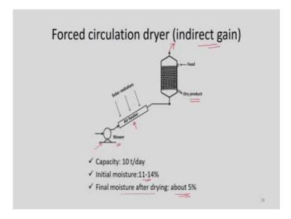
And this is one more forced circulation dryer, which is indirect gain. So, this is solar air heater, and blower is installed here. Blower blows the air, so of course we need to apply some kind of electricity to run this blower. So, air will flow through this air heater and then it will introduce here in this bed. And feeding will be done here, and then drying flow rate can be collected from the bottom of this vessel, and air can be ejected from the top.
