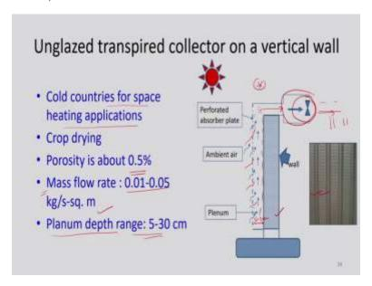
Now, let us discuss about unglazed transpired collector on a vertical wall. So, this is a vertical wall what you can see here and this is planum over which or say through which air flows and this is a perforated absorber plate. So, is ambient air will move in through this small perforations. So, one blower will be here it will suck and then air will flow and it will be distributed as per this kind of perforation devices or say ducting.
