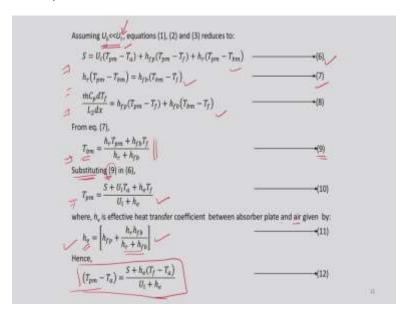
Now, assuming  $U_b$  is very, very less compared to  $U_t$ . So, this  $U_t$  is very, very high because to reduce the heat loss sufficient insulation is provided from the bottom. So, because of that this  $U_b$  can be neglected compared to  $U_t$ . So, under the condition this original equations are reduces to S is equal to this expression and than  $h_r$  would be something like this and then finally, this last expression.
