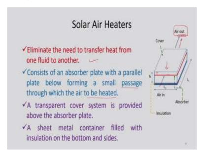
So, as far as solar heating is concerned, so, what are the different components of a solar air heaters? One glass cover at the top, then we need to have an absorber plate and then that through which air flows. So, this may be the inlet of the air and this may be the outlet of the air from where we can collect the hot air and use it for applications and also we need to provide sufficient insulation to reduce the heat losses which is generated inside the air heaters.
