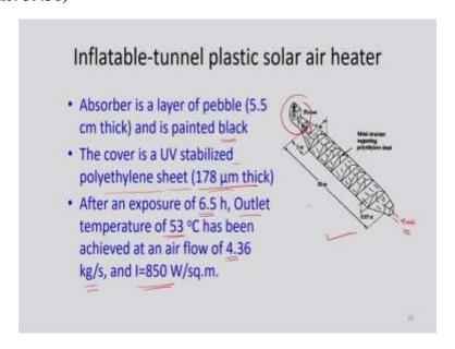
And one more solar air heater what you can see this is nothing but inflatable tunnel plastic solar heater. So, this is a blower, air is supplied from this blower and there are a number of trays where raw materials can be kept and drying can be done and this is the exit part. So, you can see length is about 50 meter people have made and this width is about 5 meter. So, this absorber is a layer of pebbles and is painted black.
