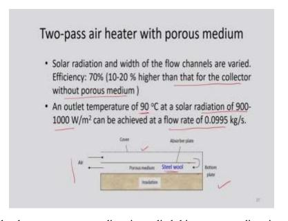
So, again here what happens porous medium is applied this porous medium is nothing but some kind of steel rules to increase the absorption of solar radiation so, that efficiency can be maximized. We have glass cover and then absorber plate and then we have bottom plate. So, this solar radiation and width of the flow channels are varied and efficiency was found to be 70 % which is 10 to 20 % higher than that of the collector without porous medium. So, in this kind of
