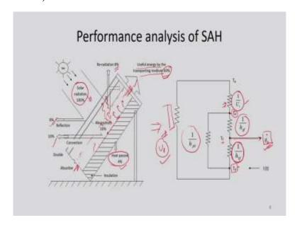
So, this slide, shows the energy flow of a solar air heater. So, here if we use double cover here, then solar air falls here through this glass cover and it is received on the absorber plate. So, energy is received here and then it is transferred to the fluid. So, as you can see if we consider this 100 % energy is coming from the solar and then some of the energy is absorbed here in the absorber itself.
