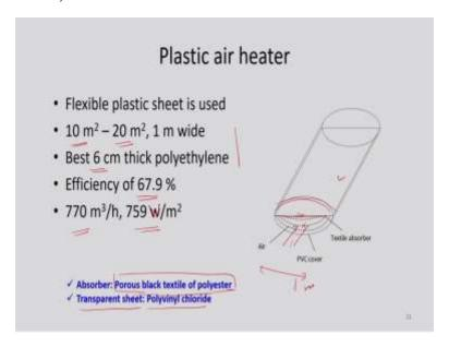
And there are certain air heaters called Plastic air heaters. So, in those kind of configurations, the absorber plate like porous black textile of polyester is used as absorber plate and for transparent
