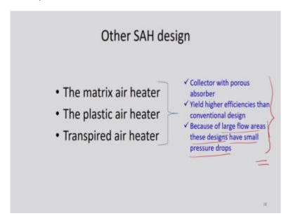
Now we will discuss some of the other solar air heater designs mostly Matrix air heater, the plastic Air heater and Transpired air heater. In all the 3 cases, collector with porous absorber plates are used and it yields higher efficiency than conventional design because of large flow areas these designs have small pressure drops. So, these are very, very important aspects of a solar air heater.
