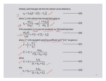
Now, similarly useful heat gain rate from collector can be calculated by using this expression where  $F_R$  is the collector heat removal factor. So, this expression is something like this which is similar to the liquid fluid plate collector what we have derived in the last class. So, if the assumption  $U_b$  is very, very less compared to  $U_t$  was not considered then equation 16 would have been something like this.
