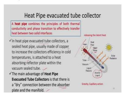
So it is seen that heat pipe technologies are used in evacuated tube collectors. What is heat pipes? Heat pipes is nothing but a heat exchanger which combines the principles of both thermal conductivity and phase transition to effectively transfer heat between two solid surfaces. So what happens if we consider this configuration. So fluid is here in this tube when solar radiation is exposed here, then this fluid will be evaporated.
