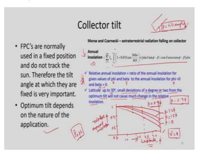
Now, let us discuss something about collector tilt. So at what angle we need to maintain for maximization of solar radiation absorption in the collector system. So what does it mean, if we make this kind of collector, we have to maintain some kind of  $\beta$ , this is nothing but tilt. So tilt angle. So this tilt angle is very, very important and this is a location specific and then time specific. So these FPCs are normally used in a fixed position.
