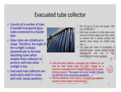
This evacuated tube collector consists of a number of rows of parallel transparent glass tubes connected to a header. So these are the headers and these are the tubes through which heat transfer fluid flows. These glass tubes are cylindrical in shapes, as you can see here, therefore, the angle of the sunlight is always perpendicular to the heat absorbing tubes which enables these collectors to perform well even when the sunlight is low.
