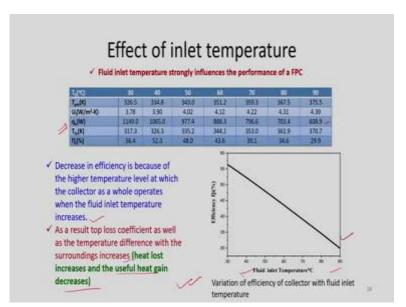
So which shows the effect of one of the most important operating parameter called temperature. This fluid inlet temperature strongly influences the performance of a flat plate collector. As you can see here, as the fluid inlet temperature increases, this efficiency is decreases. So this can be seen in this plot also. This plot shows the variation efficiency with respect to the increase in fluid inlet temperature. And other values can also be seen.
