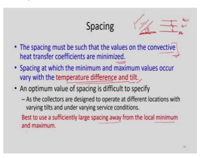
Now, let us move to the spacing between the covers. So maybe absorber plate is here, Abs, then we have glass cover 1,  $G_{C1}$ , maybe  $G_{C2}$ . So this spacing is also very very important. This spacing must be such that the values on the convective heat transfer coefficients are minimized, this is very very important. The spacing at which the minimum and maximum values occur vary with the temperature difference and tilt. So this temperature difference between this cover system and the tilt.
