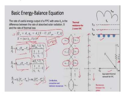
See now we know how to develop an energy balance equation. So with the previous experience we can write straight way what is the energy balance equation at the absorber
