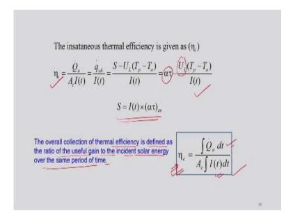
Also instantaneous efficiency is important so at any moment if we need to know the efficiency of the collector we can straight away use this expression once you know this tau alpha value and this overall loss coefficient. So this is known to us now and this overall collection of thermal efficiency is defined as the ratio of useful gain to the incident solar energy over the same period of time.
