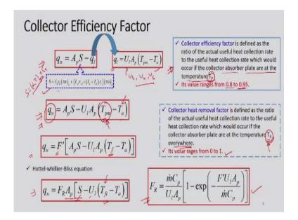
Now let us understand how this  $q_u$  are related with F' which is nothing but collector efficiency factor and an  $F_R$  which is nothing but collector heat removal factor. So already we know this expression for useful heat gain  $q_u = A_p S - q_l$  which is nothing but the losses and  $S_R$  is a function of many variables, but we can simplify  $S = (\tau \alpha)_{av} I_T$  that also we can write or we can very precisely we can use this expression and  $q_l = U_l A_p (T_{pm} - T_a)$ .
