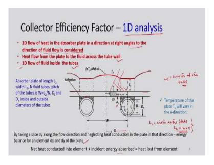
So now let us derive the expression for collector efficiency factor. So we adopt the methodology of 1D analysis or one-dimensional analysis. So in the first approach is one-dimensional flow of heat in the absorber plate in a direction at right angles to the direction of the fluid flow is considered and second consideration or second approach is the heat flow from the plate to the fluid across the tube wall and third approach is one-dimensional flow of fluid inside the tubes.
