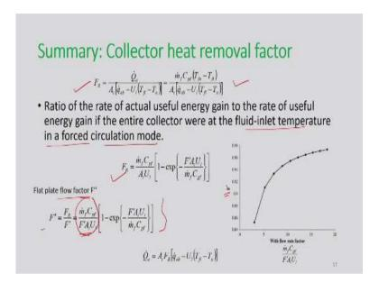
So if we summarize about collector heat removal factor so already we have defined how this  $F_R$  can be calculated and which is the ratio of the rate of actual useful energy gain to the rate of useful energy gain if the entire collector were at the fluid inlet temperature in a forced circulation mode. So this is the expression for  $F_R$  and also sometimes we can define a term called flat plate flow factor.
