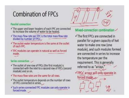
Now we will learn something about combination of flat plate collectors. There might be some cases when we need to connect the flat plate collectors in series or may be in parallel or may be both means series and parallel. So in case of parallel connections, the upper and lower headers of each FPC are connected to increase the volume of the water to be heated. The mass flow rate per FPC is the total mass flow rate divided by the number of FPCs.
