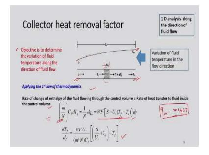
Now come to the analysis part for collector heat removal factor. So in this case also one dimensional analysis along the direction of the flow will be considered. So objective is to determine the variation of fluid temperature along the direction of fluid flow. As we have discussed the temperature variation so it goes something like this so this is an inlet of the fluid and this  $T_{\rm fo}$  is the outlet of the fluid temperature.
