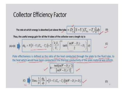
Now the rate at which energy is absorbed just above the tube also we know. So  $D_o$  is the outer diameter of the tube and this expression is known to us. So we can straightaway use it for calculation of rate at which energy is absorbed in the tube, just above the tube. So if we add this two expression this equation B expression and then equation A expression. So what we will have dq is equal to N multiplied by this expression.
