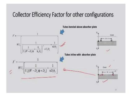
Now let us see what happens if the configuration changes. So this expression is for the tube bonded above the absorber plate so you can see the cases what we have derived just now that was for the tube which is attached below this absorber plate. Now if you see the case when this tubes are attached above the absorber plate then expression will be something like this and sometimes this inline configuration are also used in absorber plate.
