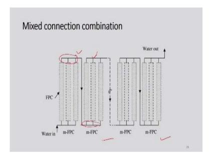
And in case of mixed connections we will have this kind of configurations. These tubes are connected in parallel again these are connected in series. This three are connected in parallel and then these are connected in parallel but know these shapes, this one and this one are connected in series so in order to get the desired temperature and mass flow rate. So this kind of configurations are really applicable in community places like may be hostels or may be in apartments.
