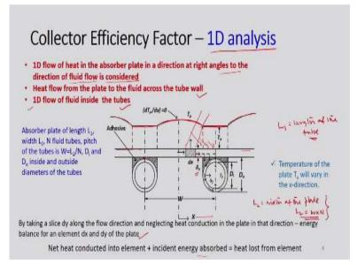
So now if we write the same expression again. This net heat conducted into the element plus incident energy balance minus heat loss from the element is 0. So what is the net heat conducted into the element? So we can use this expression for conduction and then amount of incident energy absorbed we can write  $S \times dx \times dy$  this is the area because we have considered this small segment so this is dx along this and then this is dy.
