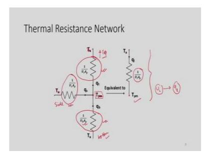
So, before we start the top loss coefficient let us understand this thermal resistance network. So, here what happens if we consider this is the plate, absorber plate at temperature  $T_{pm}$  and this is at ambient in all the cases it is ambient, this is towards top, top, this is side and this is bottom. So, heat loss will take place from this plate to the side plate to the top, then this plate to the bottom. So, these are the thermal resistances. So, we can express in terms of thermal
