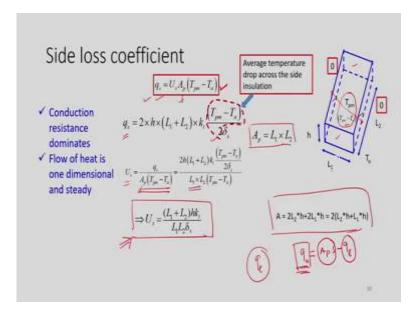
So, let us learn how to calculate side loss coefficient. So, side loss coefficient is estimated based on convection and conduction heat transfer. So, let us learn how to calculate side loss coefficient. So, this side loss coefficients can be estimated by considering both conduction and convective heat transfer. So, here also conduction resistance dominates and the flow of heat is 1 dimensional and steady. As we know  $q_s$  can be expressed something like this,  $q_s = U_s A_p (T_{pm} - T_a)$ .
