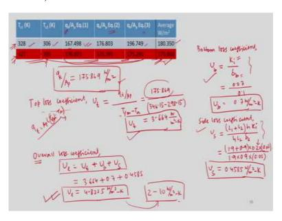
So, if 328 was the first assumption for  $T_{c1}$  and 306 for  $T_{c2}$ , then by using the equation 1 we will get this value, 167.498. And by using equation 2 we get 176.803, and by using equation
