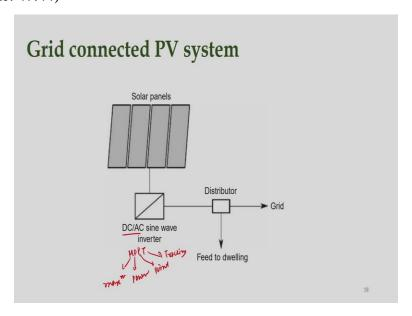
So, here it is shown about grid-connected PV system, in the grid-connected PV systems we will have modules which will be placed on the rooftop of a building and then we have to have a inverter to convert direct current to alternating current and nowadays one more very important component is called maximum power point tracking, so this tracker is introduced in the inverter itself.
