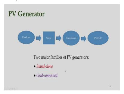
So, as far as PV generator is concerned it has got different components like we have to produce the electricity then you have to store it and then transform it and then finally we have to provide the power. So, this is how a PV generator works and there are two primary families of the PV generator, one is stand-alone system and the other one is Grid-connected system.
