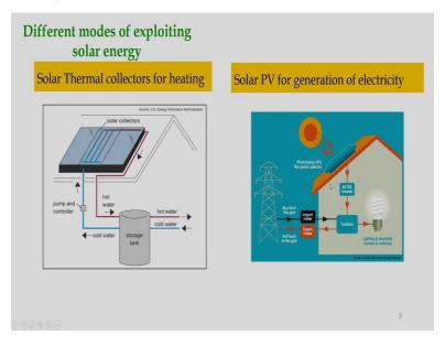
Now, this slide shows about solar thermal collector for heating as you can see in order to generate the heat energy we need to have a thermal collector where solar radiations falls and then this solar radiation is converted to some kind of heat energy and that heat energy can be stored whenever required and that energy can be used as per the requirement. And this other part of the slides shows the solar PV for generation of electricity.
