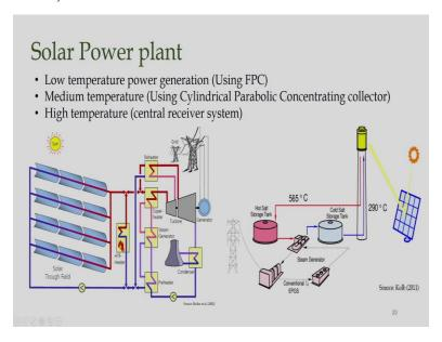
So, now come to the solar power plant, so what are different solar power plants we can make? Say low temperature solar power plant using flat plate collectors as I say, this efficiency of the conversion is very very less, so when we concentrate about low temperature power generation system. And when we move to medium temperature power plant, we use cylindrical parabolic concentrating collectors, like temperatures up to 400 degree C. And finally when we
