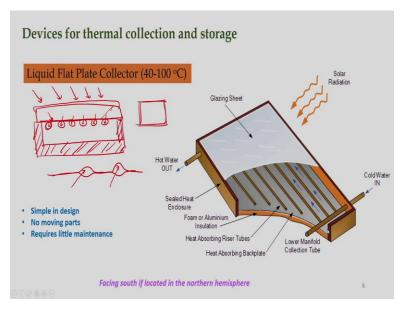
So, this slide shows about liquid flat-plate collectors. So, here what happens, when we talk about the primary component of a liquid flat-plate collectors, this component is the primary component where we will have a glass cover here and then we have a absorber plate, so this glass has to be transparent enough so the solar radiations when it falls it has to reach to the surface of the absorber plate.
