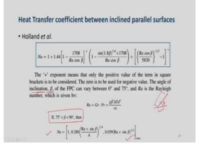
So, this is one more correlations developed by Holland et al. So, he has also suggested some kind of range with  $\beta$ , so this  $\beta$  is inclination. So, like this flat plate collector some inclination is maintained. So, this inclination we have to consider, based on this inclination we can use this correlation, if its value is between 75 to 90 then we can go for this. So, there are other conditions we have to know consider for selecting these correlations as well.
