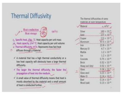
So, one more term we need to define here is a thermal diffusivity which is defined as heat conducted to the heat stored and this is mathematically represented by  $\frac{k}{\rho C_p}$ . So, Cp is specific heat and  $\rho C_p$  is the heat capacity, you can see the difference in unit J/kg °C then J/m<sup>3</sup> °C and this thermal diffusivity is represented by m<sup>2</sup>/s, which represents how fast the heat diffuse through a material.
