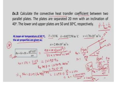
So, let us take a small problem to strengthen the understanding of what we have discussed in the last 2 slides. So, we need to calculate the convective heat transfer coefficient between 2 parallel plates. So, maybe we have to draw these 2 parallel plates and it is separated by 20 mm gap is there in between these 2 plates and it is inclined at 40 degree and upper plate is at
