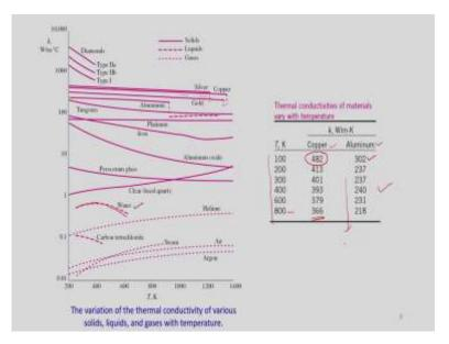
So, this figure shows the variation of thermal conductivity of various solid liquid and gases with temperature. So, as temperature increases as you can see, some of the materials so, for example, water it first increases then it decreases with increase in temperature. And for example, silver with increase in temperature it is decreasing. And this table shows the comparison of thermal conductivity of 2 different materials copper and aluminum.
