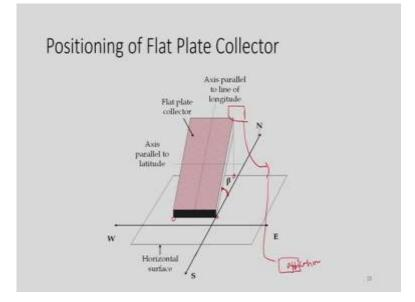
How to position a flat plate collector? So, as we know this is North, South, East and West and we have to install the flat plate collectors towards facing South or due South. So, that we can get maximum exposure to the solar radiation. So, this is the collector and we need some kind of frame to hold the structure, and we need to do some kind of civil work here to install and then we can collect the hot water from the storage bin here.
