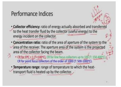
Now, there are 3 primary performance indices in case of flat plate collectors. These are collector efficiency, concentration ratio and temperature range. So, what is collector efficiency? It is defined as the ratio of energy actually absorbed and transferred to the heat transfer fluid, by the collector. So, this is nothing but useful energy to the energy incident on the collector.
