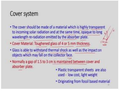
Now, let us see about cover system. The cover should be made of a material which is highly transparent to the incoming solar radiation and at the same time opaque to the long wavelength re-radiation emitted by that absorb plate. So, what I say, so this is the glass cover and then we will have this absorber plate. So, when it strikes, then some of the radiation goes back. So, this cover system has to be designed in such a way that this radiation know should be minimized.
