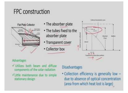
Now come to the construction of a flat plate collector. So, as far as construction of a flat plate collector is concerned, it has got 4 primary components, that is the absorber plate, then tubes fixed to that absorber plate, transparent cover, then collector box. Let us have a look on the sectional view of the flat plate collector. So, this is the outer side and here the top side will have glass cover.
