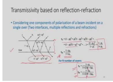
Now in continuation, the considering one component of polarization of a beam incident on a single cover. So, here only single cover is used. So, this as the whole this is a glass. So, there are 2 interfaces, interface 1 and interface 2 and there are multiple reflections will takes place. So, if we consider a beam of light, when it strikes on the interface 1 it is reflected, some
