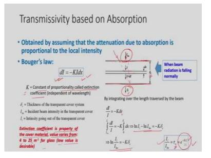
So, now, come to the transmissivity based on absorption. So, this is obtained by assuming that attenuation due to absorption is proportional to local intensity. So, which law tells us about this, it is a Bouguer's law. So, this is something like dI = -KIdx. If we consider this configuration where normal radiation is falling perpendicular to this plate, then what happens?
