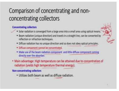
Now, if we briefly compare between concentrating type and non concentrating type collectors, then what are the differences. So, under concentrating type collectors, this solar radiation is converged from a large area into small area using optical means. So, this will be something like, we will have this large area and absorber will be here, solar radiation will fall here and it will reflect here. So, this part is absorber, and this will reflect, a reflector.
