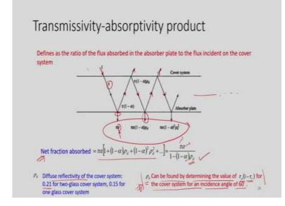
Now, let us also learn about transmissivity absorptivity product. So, which defines the ratio of flux absorbed in the absorber plate to the flux incident on the cover system. So, if we consider a beam of light and it transmitted through this cover system and maybe this  $\tau$  what we have calculated now, this  $\tau$  will introduce here and it will strike on the absorber plate. Once it strikes on the absorber plate what happens it is reflected some component will be absorbed here.
