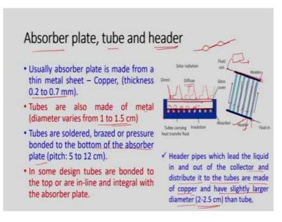
Now, let us have a look about the components. So, primary component is absorber plate then tube, then we need header. So, in this figure this is an absorber plate and these are the tubes through which heat transfer fluid flows and these are soldered here, in this tube. There are different configurations, sometimes we can have this kind of configurations, then we can get this kind configurations and there are different kinds of configurations are available.
