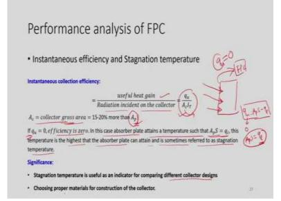
Now, we must know two important parameters, one is instantaneous collection efficiency and other one is stagnation temperature, they are related. So, how do you define instantaneous efficiency? It is useful heat gain as I have discussed this issue in the earlier slides. Useful heat gain to the radiation incident on the collector which is nothing but  $\frac{q_u}{A_c I_T}$ . So, here we have used A<sub>C</sub> as I said this collector area is 15 to 20 percent more than A<sub>P</sub>.
