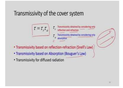
Now, this transmissivity of the cover system. So, we are talking about this cover system only. Suppose to glass covers are here, so glass cover 1 glass cover 2. So, we need to see how these radiations are behaving and what will be the transmissivity of the cover system. So, without knowing this transmissivity we cannot calculate this S or amount of flux received by the absorber plate. So, this  $\tau$  is a function of  $\tau_r$  and  $\tau_q$ . What is  $\tau_r$ ?
