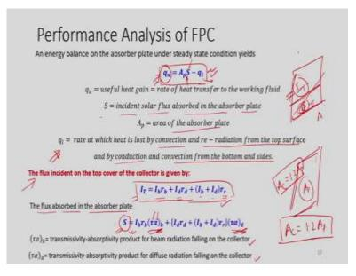
Now, come to the performance analysis of a flat plate collector. So, while analyzing the performance, we must pay attention to the energy balance on the absorber plate under a steady state condition. So, if we are interested to develop this energy balance on the absorber
