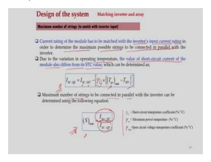
So now, let us use this current rating, okay. This current rating of modules has to be matched with the inverter input current rating, okay in order to determine the maximum possible strings to be connected in parallel. So, so far what we have discussed, the number of modules to be connected in series, okay, minimum number of modules to be connected in series and maximum number of modules to be connected in series.
