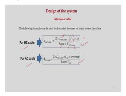
Now, we need to pay attention about the cables, right because this cable also consumes huge amount of power and cost, okay. So, to determine the cross-sectional area of DC cables we can use this equation,  $\rho$  is the resistivity, I is the know, current flowing through this circuit and this is cable length and losses will be there. And we already know  $V_{MP \ string}$ , okay and for AC cable these equations are used, okay. Of course power factors are need to be multiplied.
