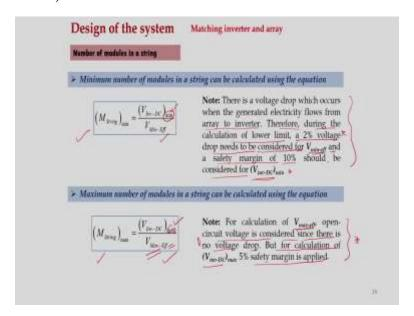
So now, let us know how to calculate this M string that is minimum number of modules in a string, okay. So, by using this equation we can calculate the minimum number of modules in a string, okay or minimum number of modules which can be connected in series, right. So, for this we need this inverter input voltage and then minimum effective voltage, okay which already we have discussed, okay.
