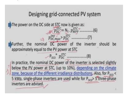
So, the power on the DC side at standard test condition is given by something like this, okay. So under test condition it will be something like this, okay, which is equal to  $N_T \times p_{MPP}^{STC}$  okay.
