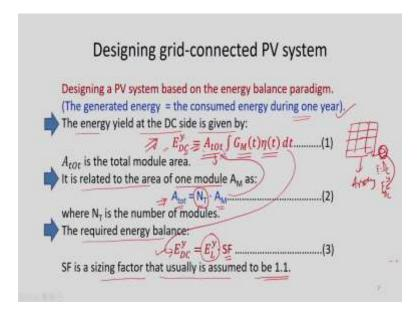
Now, come to the designing of grid connected PV system. We apply the principle of energy balance paradigm. So, here what happens, the energy which is generated by the PV arrays has to be equal to the consumed energy during one year. So, this paradigm is normally applied for designing a grid connected PV system.
