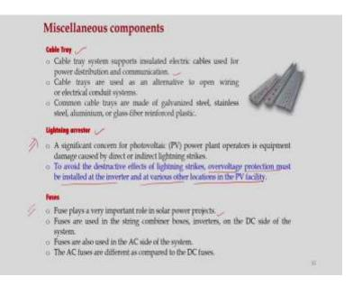
And of course, we need cable trays for installing those PV modules in this grid connected system, this cable tray system supports insulated electric cable used for power distribution and communication. So, as you can see it is something like this kind of brackets are used and then these are holes where in order to tighten the system so nut bolts are provided and then that will tighten the entire PV system.
