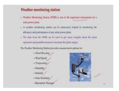
And also for this kind of PV systems we need weather monitoring stations, this weather monitoring station is one of the important instruments required for a grid connected PV system, so what information we normally get from this weather monitoring stations? So, we get wind directions, wind speed, temperature, humidity, rainfall, solar radiation and barometric pressure.
