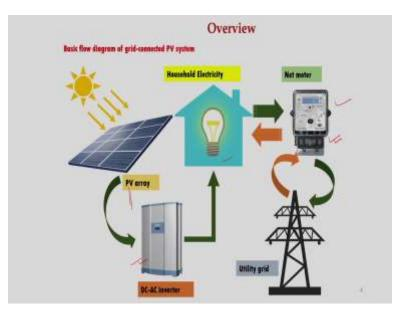
So, now see the basic flow diagram of a grid connected PV system. So, we have sun, so electromagnetic radiation will come and strike on the PV surface and then we can generate DC current, so then that has to be converted to alternating current by using an inverter, so we need an inverter to convert DC current to alternating current, then that can be connected to some load, this is called AC load and if we have generated more energy then through meter we can give it to the utility grid.
