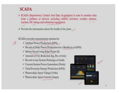
And also we need to have a SCADA system for this kind of grid connected PV system. So, what does this SCADA stands for? This is something like Supervisory Control and Data Acquisition and this is used to monitor data from a plethora of devices including meters, inverters, weather stations, trackers, DC strings and substation equipment.
