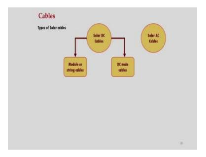
And primarily these cables are classified into two categories DC cables and AC cables, so DC cables again we have modular string cables and DC main cable.
