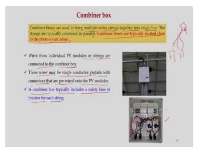
Now, let us see what is combiner box, this combiner box are used to bring multiple series string together into a single line, know already we know these modules and that has to be connected and finally it will come as a single wire and where it will be connected? It will be in combiner box. The strings are typically combined in parallel, this combiner box are typically located close to the photovoltaic array, so this we must know.
