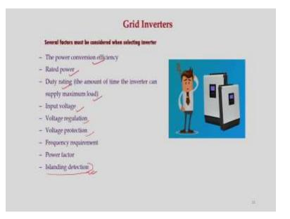
So, there are some factor which must be considered when selecting an inverter. So, what are those factors? Like power conversion efficiency, rated power then duty rating which means the amount of time the inverter can supply maximum load, then input voltage, then voltage regulation, voltage protection, frequency requirement, power factor and islanding detection, this is very, very important. So, we will discuss what is islanding and islanding detection.
