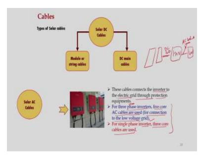
And let us learn what is solar AC cables. Already we know once we have inverter so maybe what we can consider here, so we have these are maybe modules, modules and then we have inverter, then we have cables and then it goes to the load or maybe grid. So this cable is DC cable, this DC cable and this is AC cable, so what we are talking about this AC cable.
