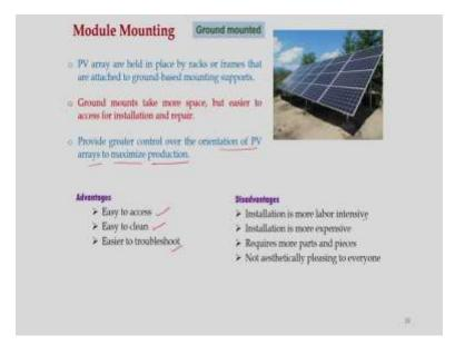
So, for ground mounted system, as you can see we need to have a strong structure to hold this entire PV panels and other components, then how we can define it? This PV array are hold in place by rack or frames that are attached to ground based mounting supports, so again we have to do something here civil work, so cement and other thing you need to apply then we have to have a pole then strong foundation needs to be made so that involves lot of cost.
