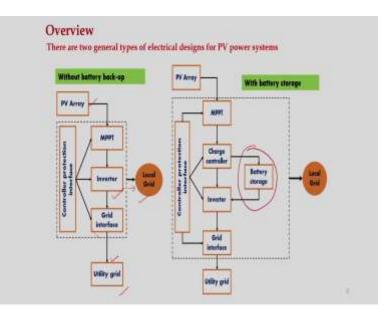
So, there are two general types of electrical designs for PV power stations and the first design is without battery backup and second design is with battery backup. So, components already it is known to us now PV arrays we need then we need MPPT because we need to operate at maximum power point by using the electrical or mechanical system and then we need to have inverter to convert direct current to alternating current and then grid interface.
