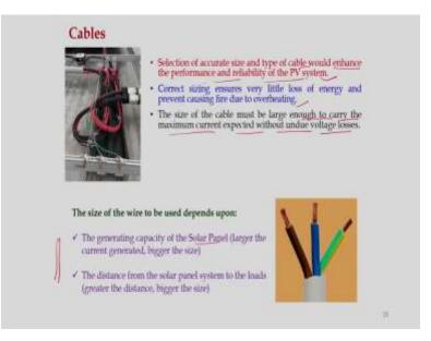
So, now let us learn something about the cables, the kind of cables used in grid connected PV system. So, this selection of cable plays a key role in the proper functioning of a grid connected PV system. So, this selection of accurate size and type of cable would enhance the performance and reliability of the PV system, the correct sizing ensures very little loss of energy and prevent causing fire due to overheating.
