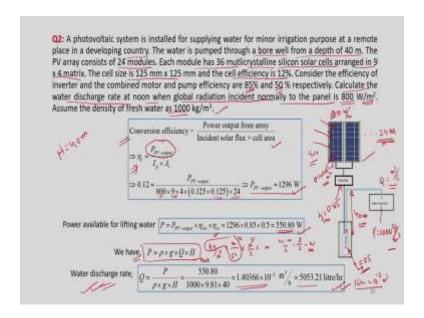
So, let us take a small exercise to understand this properly. So, this problem goes something like this. A photovoltaic system is installed for supplying water for minor irrigation purpose at a remote place in a developing country. The water is pumped through a bore well from a depth of 40 meter, so head is given as 40 meter, 40 meter head.
