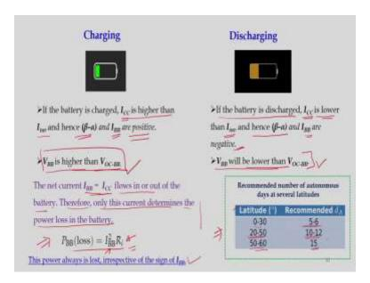
So, there are two conditions, already we know charging and discharging. So in case of charging if the battery is charged then  $I_{CC}$  is higher than  $I_{inv}$ , that we must know. So, this  $I_{CC}$  is higher than  $I_{inv}$  and hence,  $\beta - \alpha$  and  $I_{BB}$ , this current flowing through this battery bank are positive. So,  $V_{BB}$  is higher than  $V_{OC}$ , so we can see why  $V_{BB}$  is higher than  $V_{OC}$  by analyzing the solution of the quadratic equation.
