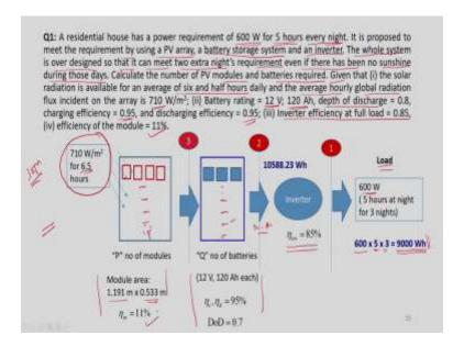
So, let us take an example to understand how we can design a standalone PV system. So, this example goes something like this. A residential house has a power requirement of 600 watt for 5 hours every night and it is proposed to meet the requirement by using a PV array, a battery storage system and an inverter. The whole system is over designed so that it can meet two extra nights requirement even if there has been no sun shine during those days.
