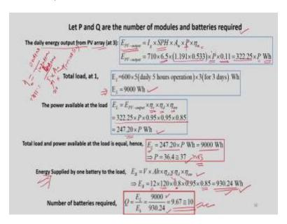
So, let us consider P and Q are the number of modules and batteries required to run the system. So, now what we will do? We will start with this supply part, like daily energy output from PV array at 3, if we go back here.
