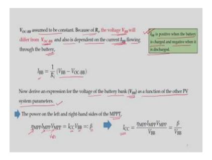
So, now as we said this  $V_{\text{OC-BB}}$  assumed to be constant for our analysis because of this  $R_i$  the voltage BB that is a battery bank voltage will differ from this open circuit battery bank voltage and also is dependent on the current  $I_{\text{BB}}$  the amount of current that is a battery bank current flowing through the batteries.
