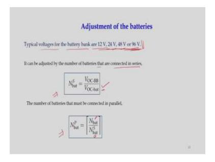
Now, we must know the number of batteries to be connected in series and number of batteries are to be connected in parallel. If we consider a typical voltage for battery bank maybe 12 volt, 24 volt, 48 volt and 96 volt these are specified in case of lead acid batteries.
