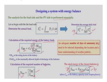
Now, let us design a standalone PV system with energy balance. So, the analysis for load side and the PV side is performed separately, so first let us consider the load side, then we will go for the supply side or generation side. So, if we start with the load side then first we are interested to know the annual load.
