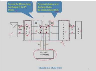
So, the power on the left and right hand side of the inverter, so if you go back to the slides you can see, so this is the inverter, so this side is how much is the  $I_{AC} \times V_{AC}$  and this side you need to consider the efficiency of the inverter, then see how it look likes.
