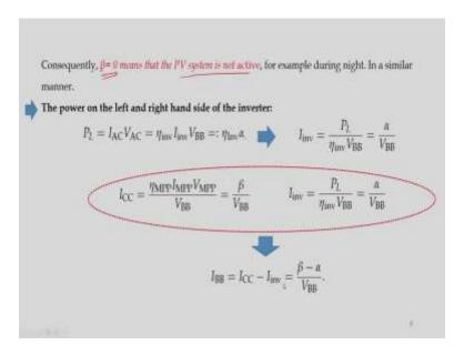
So, now let us learn more in depth, if  $\beta$  is 0 means that PV system is not active, maybe at night PV system is not active because no solar energy is there, no solar radiation is falling on the PV system. So what happens then if  $\beta$  is 0 then you can see the expressions what will happen, so  $\beta$  is 0 means no current will flow through this circuit.
