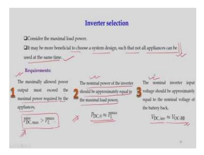
Now, very important factor is selection of inverter. So, while selecting the inverter we must be very, very particular, this inverter should meet some of the requirements. So, number one is the maximally allowed power output must exceed the maximal power required by the appliance.
