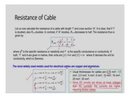
So, also we know this  $R_{cable}$  is function of row  $\rho \frac{l}{A}$  and also  $\frac{1}{\sigma}$  is  $\frac{l}{A}$  right. So, this row is nothing but resistivity and also we can express in terms of conductivity okay this is conductivity, right. Normally this I will be in meter and a is normally in millimeter okay. So, this block shows about the no values of this row for copper and aluminum because mostly copper and aluminum cables are used in applications.
