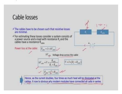
So, now, let us have a look about the cable losses okay. So, these cables have to be chosen such that resistive losses are minimal, okay. So, in order to understand this let us take an circuit which constitutes a supply voltages okay and then we have load and then maybe cable resistance are included, okay. So,  $R_L$  represents the load having resistance  $R_L$  okay and this R cable is the resistance of the cables right.
