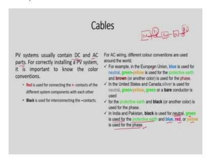
Now, we need to also learn the cables, cable plays an important role in the functioning of a PV system right. So, PV system usually contains DC and AC part as you can understand, so, when we are talking about PV modules, okay, or arrays so, power generated here will be DC then we will have okay battery we can write and maybe inverter here, okay? Then we will have AC okay.
