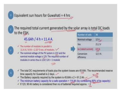
Let us move to the next step. So, equivalent sun hours if we consider a place in Guwahati so it may be four hours okay. So, required total current generated by the solar array is total DC load to
