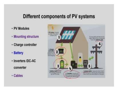
So, different components of a PV systems are PV modules which is the primary component then mounting structures then charge controller, battery, inverter, then DC AC converter and cables. So, as you can see here in the figure, so, PV modules are installed on the rooftop okay. So, this PV array converts sunlight into direct current right and we need to have a charge controller to protect the battery from the overcharging, right.
