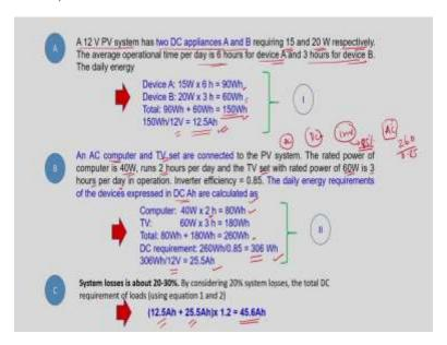
So, the example goes something like this a 12-volt PV system, we are considering very basic PV system has two DC appliances A and B. So, two DC appliances we are considering maybe A and B that may be anything requiring 15 and 21 watt respectively okay, the average opertional time per day is six hours for device A and three hours for device B right.
