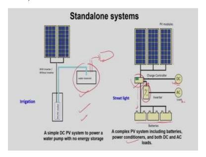
So, what you can see here, they are two configurations of a standalone system. So, first configuration where there is no charge controller and battery bank and the second configurations will have charge control and then battery banks okay. So, here this is an example of lifting water from the ground and storing in a reservoir and then finally we can use this reserve water for irrigation applications, okay.
