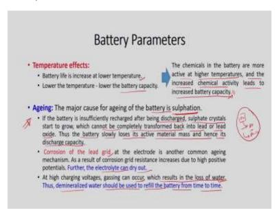
And how temperature affects the battery life. So, this battery life is increased at lower temperature okay if you can keep at low temperature or room temperature then battery life is expected to be higher and lower the temperature, lower the battery capacity again okay. So, what happens the chemicals in the battery are more active at a higher temperature okay and the increase chemical activity leads to increased battery capacity okay. So, by increasing the
