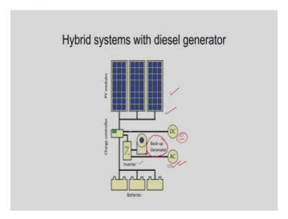
One more configuration we have, suppose in a single day we do not have enough sunlight, okay then amount of energy generation by this PV module will be very very less okay then under the conditions in order to meet the demand then we need some kind of backup system, okay. So, here what we have shown this is a generator backup system and this is coupled with that existing connections right.
