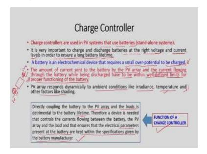
Now, let us discuss something about charge controller, which plays a key role in a stand-alone system where a battery is involved, okay. So, charge controllers are used in PV systems that use batteries okay. So, it is very important to charge and discharge batteries at right voltages and current levels in order to ensure the longer battery life time, okay.
