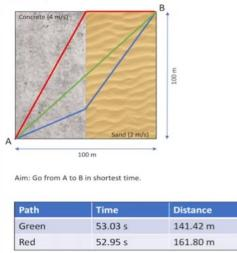
Now I will start the introduction with classic puzzle okay look at this diagram here. In this diagram it is like a big field which is 100 meters by 100 meters and on the left side of that field is the concrete and on the right hand side on the right half there is sand and there are these diagonal points which have marked as A and B and the aim is to go from A to B in shortest possible time okay. What is the catch? Catches us.
