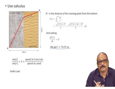
Now there is another way use calculus see since we already have figured out the nature of the path calculating the time for this path is very easy. So the path can easily be given by an integral of ds over v where ds is small length element along the path and then because the velocity is on concrete side is fixed velocity on sand side is fixed the formula can be immediately integrated to something like this.
