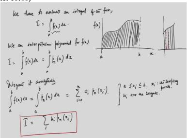
So, let us just see what we mean graphically by numerical integration so we have to evaluate an integral of the form I equal to a to b f of x dx okay. So, what it means is that let us have a f of x which is simply like this and so this is f of x versus x and said this drain or this end is a having a value x equal to a. And say we have a value which is x equal to b and we need to know by this integral what it means for this particular case is that we need to know the area under the curve.
