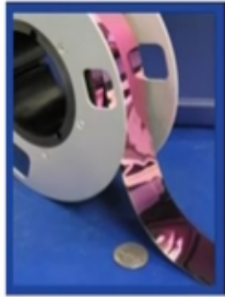
American Superconductor 2G wires: YBCO based, with Y_2O_3 nano particles for flux pinning.
