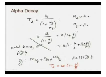
So, we have a T alpha equal to Q divided by 1 plus m alpha over my. Now if I approximate m alpha to 4 atomic units, and m y to a atomic units then this will give me T alpha equal to Q over 1 plus 4 by a, this is an approximation now I can invert this and write it as let me write it as Q 1 plus 4 over a times minus 1, and binomially expand it to get 1 minus 4 by a, plus higher order corrections order 4 by a square.
