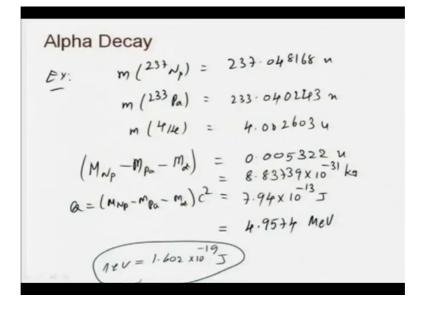
Now let us take an example, a consider the example that we have considered just now m of 237 in p is equal to 237.048168 atomic units, and mass of 233 pa is equal to 233.040243 units and mass of alpha particle is 4002603 units. So, the mass difference the mass of the neptunium minus, mass of palladium minus mass of alpha particle is equal to, you can find the difference between this and that turns out to be 0.005322 good.
