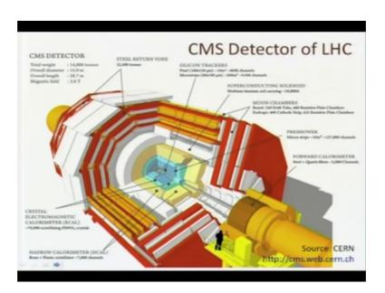
So, a CMS detector is has many different parts as you can see basically the beam pipe is at the center along the axis of this surrounding the blue of blue 2 blue arrows that we have in this picture and this is surrounded by different layers of detectives first we have what is called the silicon tracker the silicon tracker is something which actually tracks the particles it detects the particles type of the particle.
