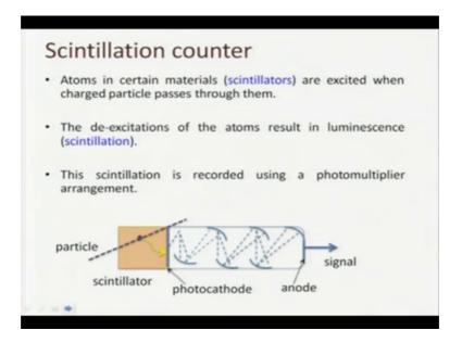
Another thing just now when we mentioned the scintillation counter. So, that is another type of detector when charged particle pass through certain materials atoms of these materials are excited these materials are called scintillators and when these excited atoms be excite there will be luminescence it will emit radiation it will emit electromagnetic radiation this is basically in the visible range and then say scintillator; this particular and this reminiscence is called scintillation.
