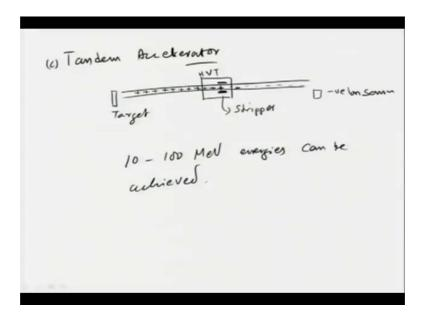
So, tandem accelerator principle is the same as the Vande Graff generator accelerator the only difference is that now you have the accelerating tube suppose you were interested in some kind of a particular positive ion; what you do is to actually generate the corresponding negative ion source ion basically I mean you can actually deposit electrons by some mechanism we will not discuss how it is done and to the items of interest and you can have the ions there indirectly negative ions.
