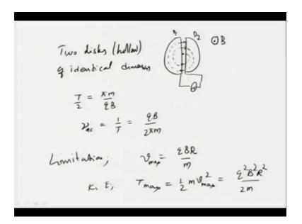
We will take 2 circular disks we will take some kind of a hollow disk and call it D one and D 2. So, let me draw that. So, this is actually a disk. So, one is D one the other is D 2. So, 2 identical 2 disks of identical dimensions say they are hollow disks of identical dimensions.
