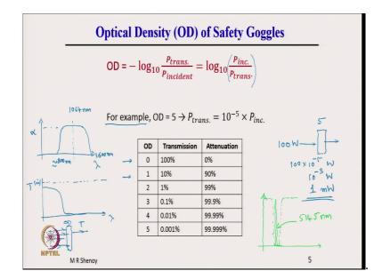
So, let me explain what is this optical density OD, because if you take a laser goggle or a eye safety wear, it is always written that OD equal to 5 or OD equal to 6, what does this OD mean? So, OD stands for optical density and it is defined as minus 10 log power transmitted divided by power incident or intensity transmitted intensity by incident intensity.
