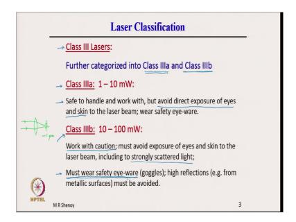
This is further categorized into class IIIa and class IIIb. I must mention that there are many other classes, classification based on various other things, but these are the broad classifications. So, class IIIa and class IIIb lasers. Class IIIa power levels in the range of 1 to 10 milli watt, again they are relatively safe to handle the normal laboratory lasers, which we use in a laboratory; a teaching laboratory are in the range of 1 to 10 milli watt.
