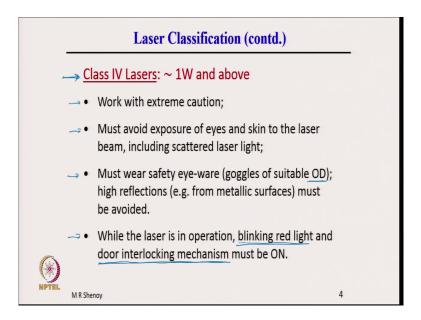
Now, let us go to the next class, which is the class IV laser. So, class IV lasers have powers of the order of 1 watt and above; all lasers with power greater than or of the order of 1 watt, sometimes even 500 milli watt is classified as class IV laser.
