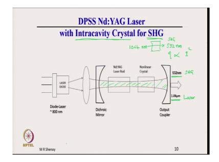
There is a Nd:YAG laser with the intra cavity crystal for second harmonic generation. The Nd:YAG laser which is shown here; if we can have an intra cavity crystal, intra cavity means inside the cavity crystal, then it can lead to efficient second harmonic generation. I will discuss this application of second harmonic generation in detail in a subsequent lecture.
