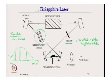
So, what is shown here is a schematic of the setup for the titanium sapphire laser. So, titanium sapphire is a tunable laser; so, this has a spectrum which is it is tunable over say tunable over approximately from 700 or 780; so in the range of 700 to 1100 nanometer, that is a very very wide range of tunability in the case of lasers.
