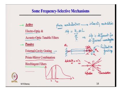
Here I finally, come to some frequency selective mechanisms. So, these mechanisms can be used to select different frequency lines or to tune the output of a laser. There are active methods and passive methods; so, active and passive methods for frequency selection. We will not go into the details, in the case of active methods usually electro optic technique or acousto optic technique which I have briefly discussed.
