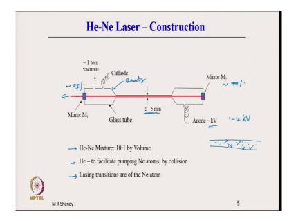
So, the schematic of the laser looks like this. So, there are two mirrors at the output end, generally the mirror reflectivities are very high. So, mirror reflectivity could be 99 percent and 98 percent or 97 percent of that order very high reflectivities. Because, the gas is a very inefficient gain medium and therefore, the mirrors must be of very high reflectivity, so that the threshold can be reached or the resonator losses can be maintained as low as possible.
