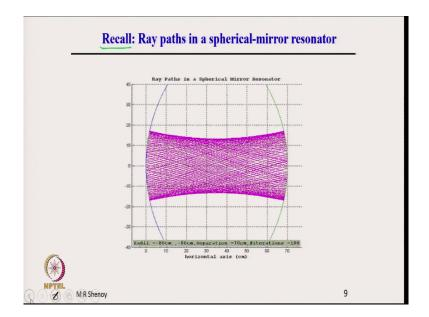
So, what is shown here is just to recall the ray paths which we had seen earlier in the spherical mirror resonator that the beam looks like a Gaussian beam which goes back and forth, when you draw the ray paths. And that is why we have shown here, a Gaussian beam which is going back and forth inside the spherical mirror resonate.
