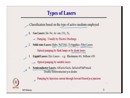
So, let us look at some of the types of laser and the classification in this case is based on the type of active medium employed. So, gas lasers first: the helium neon, argon ion, carbon dioxide, nitrogen laser and so on; all gas lasers. The active medium that is the medium which provides amplification when excited appropriately is a gas.
