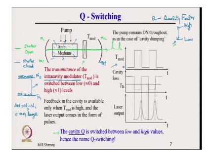
So, now let us see what is the difference between Q-switching? In the case of Q-switching, there is an external modulator, there is a modulator which is placed inside the resonator, its a intracavity modulator. In the case of external modulation, we had this modulator outside the cavity. Now, in this case, the modulator is placed inside the cavity the modulator is essentially a shutter which is open or closed.
