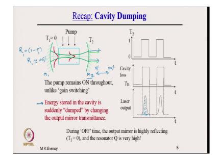
So, what is the difference between Q switching and cavity dumping. Let us have a look at cavity dumping. In the case of cavity dumping, the energy was stored inside the resonator. When the transmittance was 0, which means the reflectance of this mirror is nearly 100 percent, the energy is stored inside the resonator and when the mirror transmittance suddenly switched to 1 which means the reflectivity became 0, the laser output came as a flash from the mirror 2.
