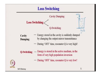
Then, we said loss switching. In loss switching there are two methods which are used cavity dumping and Q switching. In the last lecture, we discussed cavity dumping which is very easy to understand if we consider a an analogy of a bucket here with flap which could be opened so, let us say there is a flap and we could open this flap like this.
