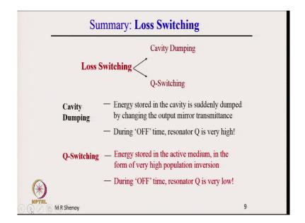
Let me summarize therefore, so, that is the summary slide which I had shown earlier. Cavity dumping energy stored in the cavity is suddenly dumped by changing the output mirror transmittance. During off time, the resonator Q is very high. Off means when there is no output that means, the reflectivity of the second mirror is almost 100 percent which means the resonator Q is very high.
