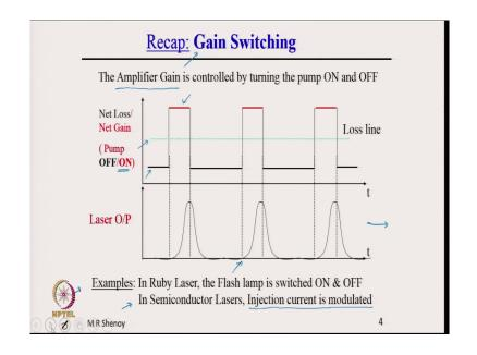
The second method which we had discussed is gain switching where the amplifier gain is controlled by turning the pump on and off. So, we have discussed this. So, what is shown here is the pump off, on. When the pump is off, pump level is off, then there is net loss in the system, this is the loss line of the cavity resonator, this is the loss in the system that is there is no gain provided by the amplifying medium.
