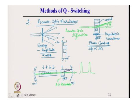
The second method which is used is by using acousto-optic modulators. The basic principle of acousto-optic modulator, there is a crystal here and you apply an RF radio frequency a RF modulator using a transducer so, this is the crystal; crystal, this is a peso electric crystal and therefore, the RF leads to mechanical waves travelling through the medium. There are compressions and rare fractions in the medium that leads to a refractive index variation along the medium.
