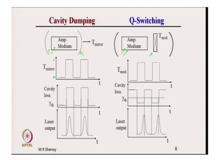
A comparison which is again shown here side by side. So, see the comparison, here the transmittance of the second mirror is what is modulated switched between 0 and 1. Accordingly, the cavity loss is switched and accordingly, we have a pulse output which comes out.
