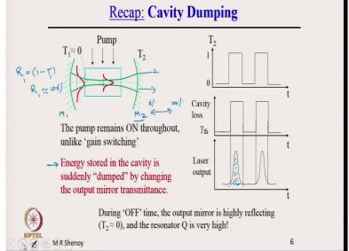
So, let us just look at the cavity dumping very quickly. So, here is the laser with the mirrors M 1 and M 2; so, mirror M 1 and M 2. M 1 has a transmission which is T 1 which is nearly equal to 0 which means the reflectivity or reflectance is equal to 1 minus T is nearly equal to 1 which means R 1 so, this is T 1 which is R 1 is nearly equal to 100 percent, the reflectivity of the first mirror is 100 percent.
