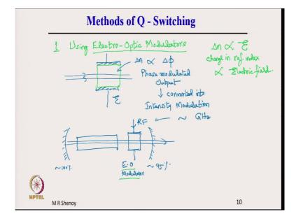
So, methods of Q-switching. There are two important methods, one is by using electro optic modulators so, using electro optic modulators. So, please recall the diagram here. So, I am referring to this modulator here. So, the modulator here could be electro optic modulator or acousto-optic modulator, these are the two popular methods of using Q-switching. So, let me discuss these in brief.
