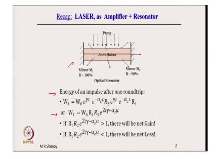
A very quick recap, laser as an amplifier plus resonator; in the last lecture, we saw how the laser, which is a oscillator is a combination of amplifier plus resonator. So, what is shown here is the laser medium, gain medium and two mirrors coated at the ends forming the resonator.
