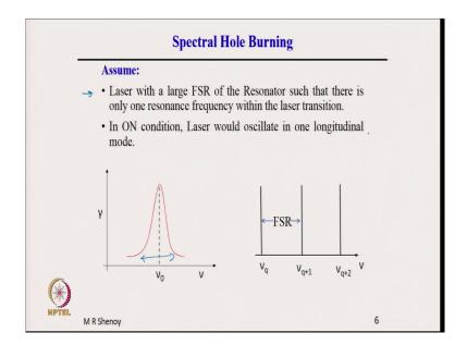
Now, assume a laser with a large FSR of the resonator; we have already discussed this that, if the FSR Free Spectral Range is sufficiently large within the laser transition or within the laser gain region, we could have only one oscillating longitudinal mode.
